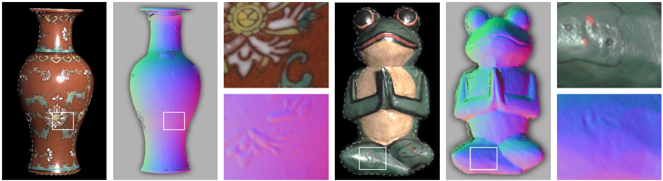
Figure 6: Normals computed from two objects with complex spatially-varying isotropic reflectance. Normals are visualized according to (r, g, b) = (\frac{n_x+1}{2}, \frac{n_y+1}{2}, n_z) . The dashed line in each reference image indicates the region shown at right.
