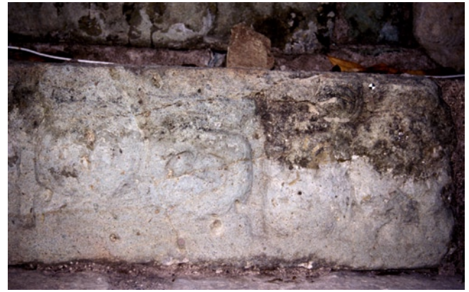
Figure 107 Treatment trial block 463, step 50, glyphs F and G, shown after the cleaning of glyph F (on the left) with water and a light toothbrushing; glyph G (on the right) has not been cleaned.
