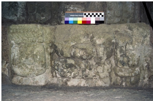
Figure 116 Treatment trial block 578, step 61. Glyph Q, on the left, is shown after reduction of previous treatments and new stabilization treatments; glyph R, on the right, shows the darkening over time of previous stabilization treatments.
