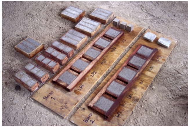
Figure 100 Cube and prism molds of trial mortars before curing.
