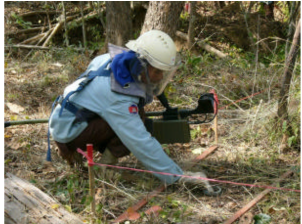
Figure 3 A CMAC deminer scanning the soil surface with the ring-magnet.
