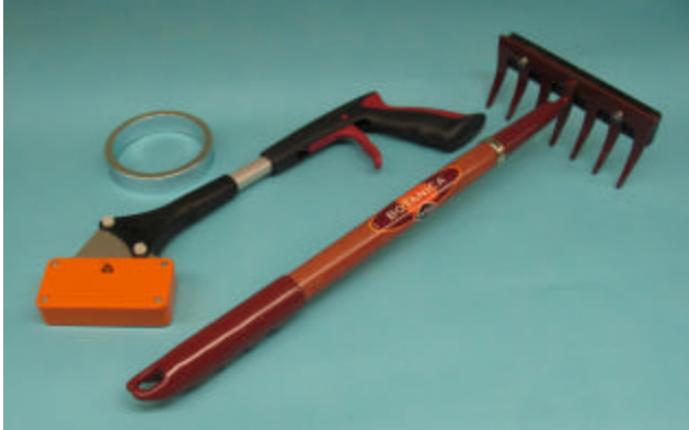
Figure 1 Three types of magnet-tools in the test: ring-magnet, Hand-Held Sweep Magnet and magnet-rake (from left to right).
