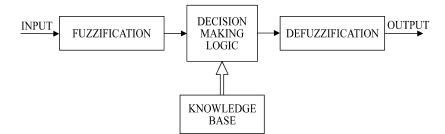
Fig. 2 Fuzzy Controller Block Diagram
