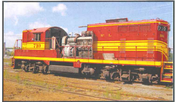
GP7 #710 in Copperhill awaiting removal of the old main generator and installation of a replacement. Photo by Mike Little.
