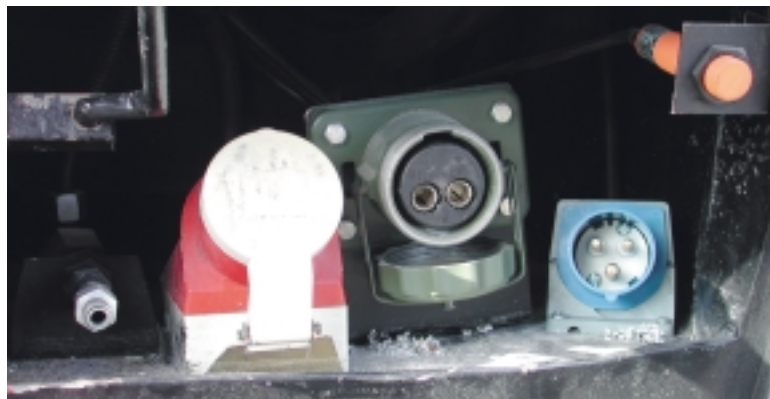
Fig. 12. Connectors for charging, heating and air during parking.
