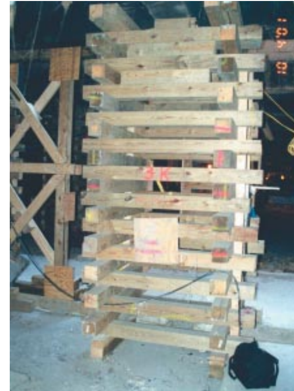
Figure 5.17 Column missing at location 3K
