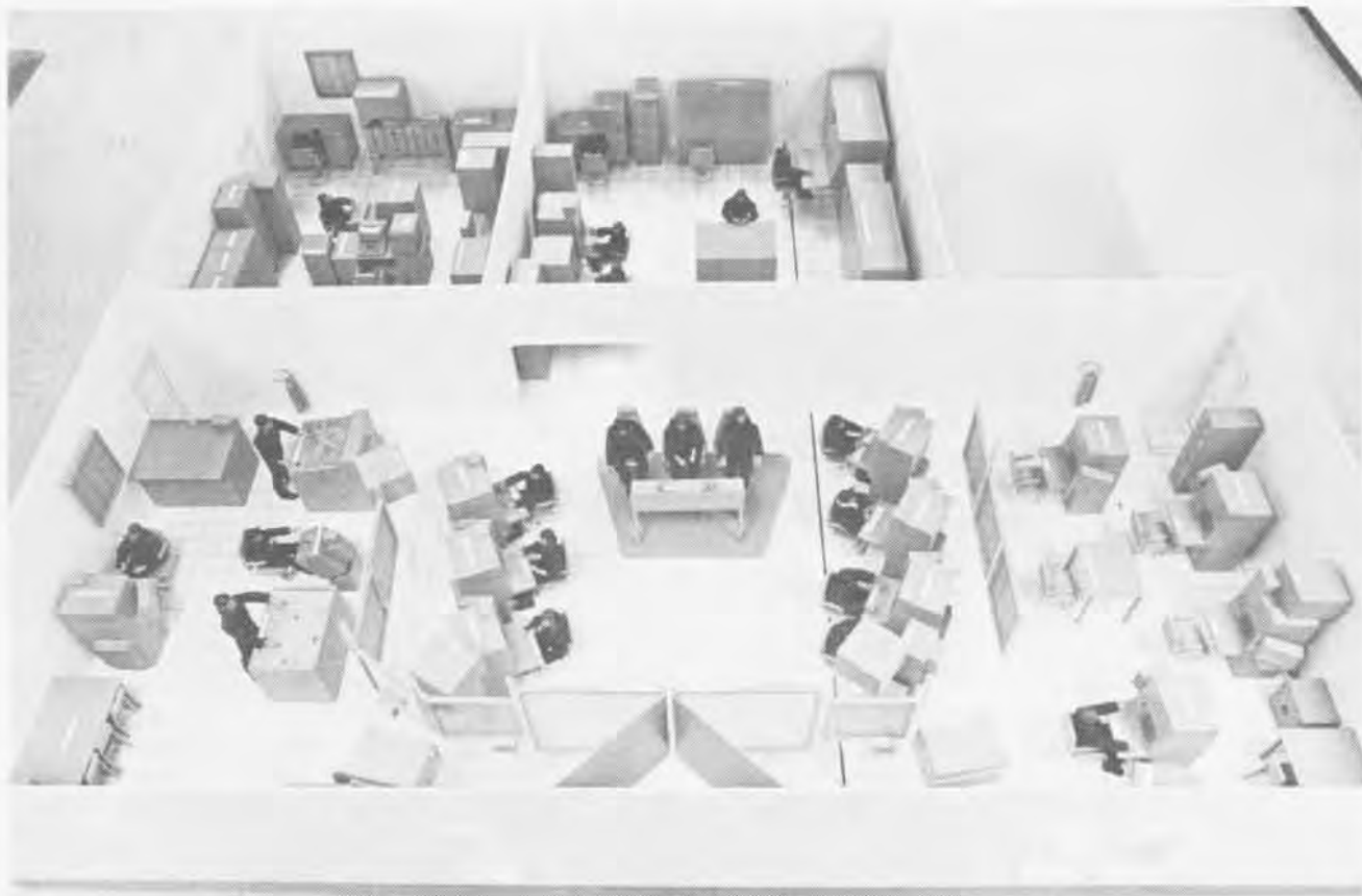
Mock-up view depicts the display and decision surface warfare and air warfare areas in the combat information center of the proposed CVV. Raytheon, a NavSeaSysCom support contractor, assembled and helped design mock-up in conjunction with the Naval Ship Engineering Center.
