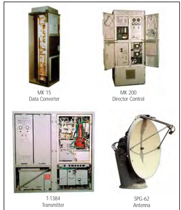
MK 99 Fire Control System Components
