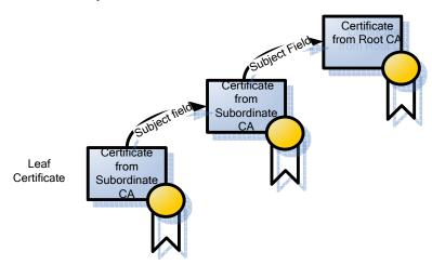
The Issuer Field of a certificate equals the Subject Field of the certificate of the issuing CA. In this way, each certificate points to the next certificate in the chain, until the path reaches a certificate created by the root CA.
