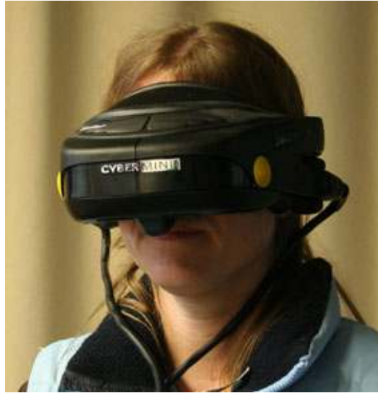
Figure 6.3: A user is pictured wearing a current generation HMD, the Cybermind Visette45 SXGA.
