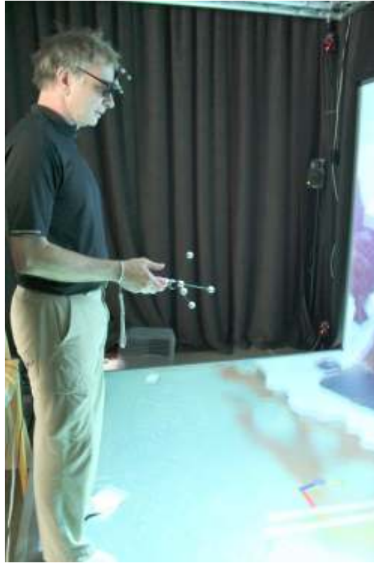
Figure 6.4: Here the user can be seen in the imveL, an L-shaped large scale projection based VR system. The system include 3D sound system and tracking via an optical tracking system.
