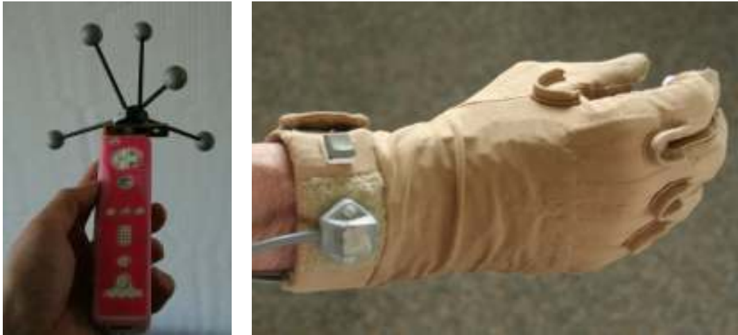
(a) A wand built from a Nintendo Wii controller with an attached optical tracking target (b) A glove input device with bend sensors and an attached electromagnetic tracking target
