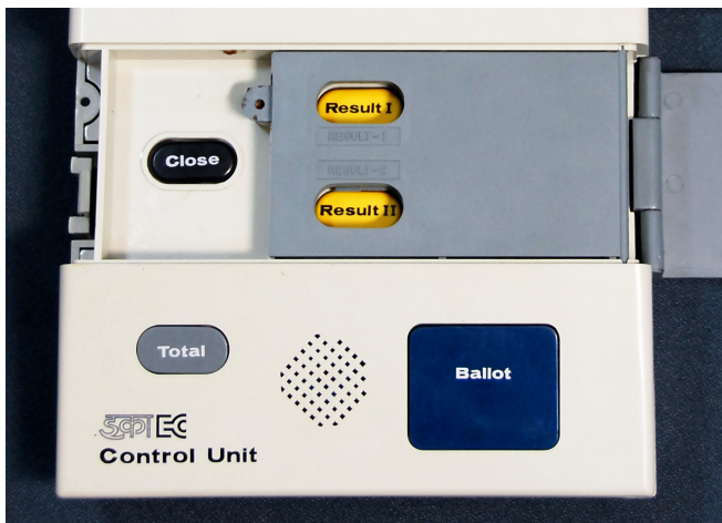
Figure 2: Counting Votes — The EVM records votes in its internal memory. At a public counting session, workers remove a seal on the control unit and press the RESULT I button ( left ) to reveal the results. The machine sequentially outputs the number of votes received by each candidate using a bank of 7-segment LEDs ( right ). Here, candidate number 01 has received 7 votes.
