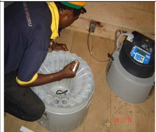
Equipment and methods used to collect high frequency (sub-daily) suspended sediment samples at 1DD1-Kikuletwa station (i.e. Node 1).
