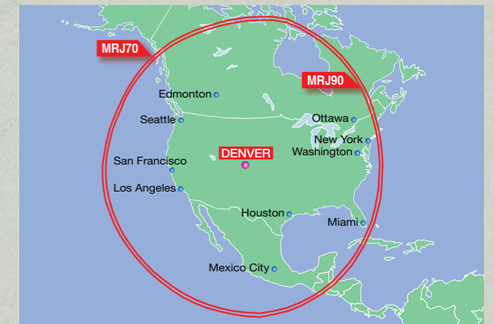
ISA, 85% Annual Wind, Alternate 200nm Payload: MRJ90 92pax x 102kg (225lb), MRJ70 78pax x 102kg (225lb)
