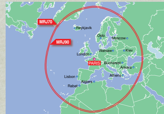
ISA, 85% Annual Wind, Alternate 200nm Payload: MRJ90 92pax x 102kg (225lb), MRJ70 78pax x 102kg (225lb)
