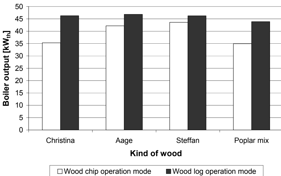
Figure 3: Average output of the boiler in kW th depending on the kind of wood and the operation mode of the boiler in a stationary operation point
