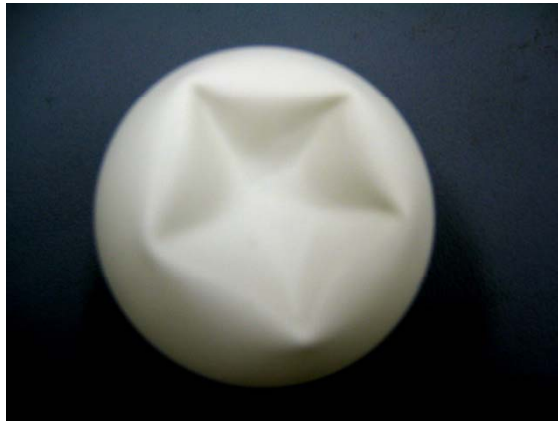
Ping Pong Ball : plastic deformation and no volume conservation
