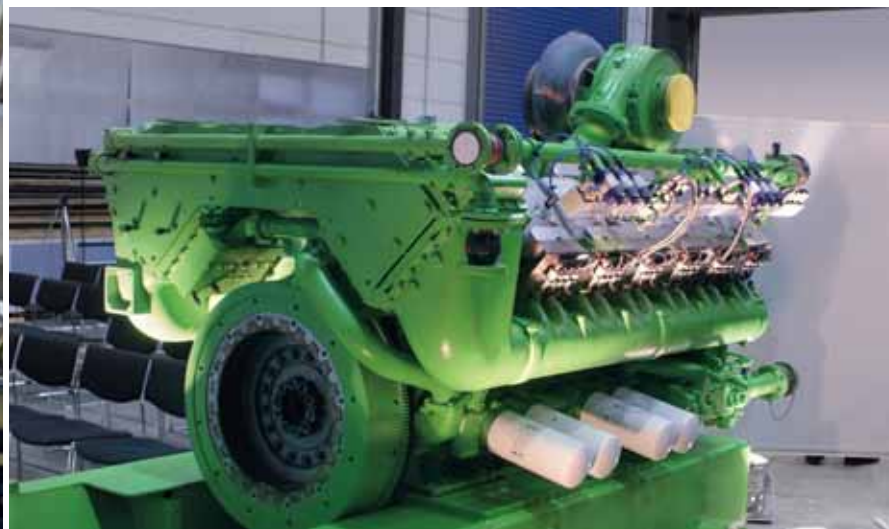
Orange Line in Philadelphia (top, right), LPG engine for remotorizing locomotives
