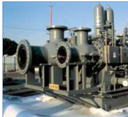
A three stage expander mounted on a single integral gear. This natural gas pressure letdown application handles 68 MMSCFD (76,000 Nm 3 /hr) and produces 5-MW of electrical power.
