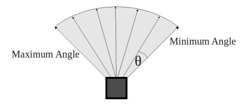
Figure 23: A laser scanner. The minimum angle is the angle of the rightmost laser scan, the maximum angle is the leftmost laser scan.  $\theta$  is the scan resolution of the laser, it is the angle between each laser scan, given in 0.01 degrees.
