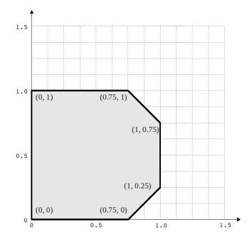
Figure 8: The basic shape we want to make Bigbob, the units on the axes are in metres.
