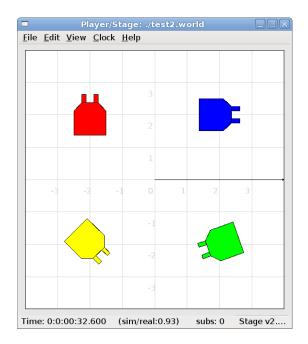
Figure 11: Starting from the top right robot and working anti-clockwise, the yaws of these robots are 0, 90, -45 and 200.
