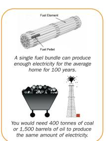
Natural uranium ore is mined in Canada. The uranium ore is converted to a yellow cake  $(U_3 0_8)$  at the mine. It is then taken to the uranium refinery in Port Hope, Ontario where it is refined to uranium oxide  $(U0_2)$ , a black powder. At the fuel fabrication plant, the powder is compressed into fuel pellets, which are then baked in an oven to harden and give them properties of ceramic material. The fuel pellets are placed into 37 fuel elements that are assembled to create a fuel bundle.
