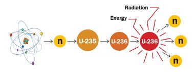
Fission occurs when a neutron strikes an isotope of uranium-235 (U-235) atom, creating the unstable element uranium-236 (U-236). The extra neutron results in the U-236 atom splitting and releasing other neutrons, energy and radiation. After moderation, the released neutrons go on to cause further fission and the cycle is repeated.
