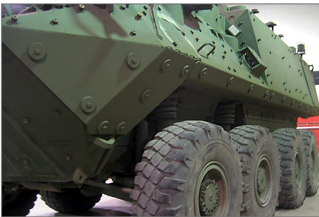
Bison with Heavy Blast-Fragments IED-Protection
