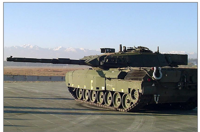
Leopard 1 with Multi-Purpose IED-Protection
