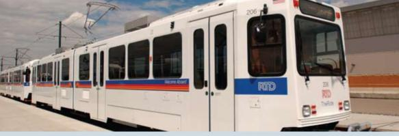
Bi-directional, six-axle, high-floor single articulated light rail vehicle constructed of low alloy high tensile (LAHT) steel, with step-wells suitable for street-level boarding.
