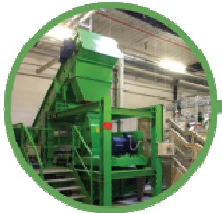
In step two, the hammermill crushes the glass further into approximately 4-5mm pieces, small enough to ensure the lamination bond is broken.
