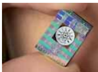
SSAC – Solid-State Atomic Clock on a silicon CMOS chip
