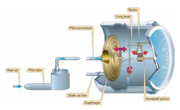
Figure 3-11. Mechanism of an Airspeed Indicator.
