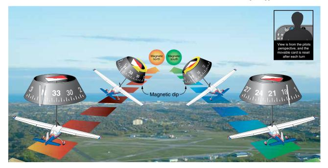
Figure 3-20. Northerly Turning Error.
