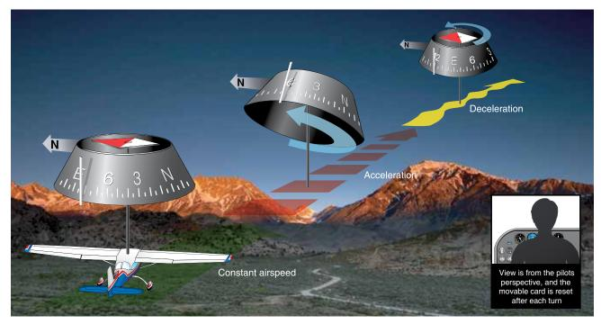
Figure 3-21. The Effects of Acceleration Error.
