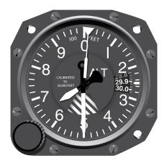
Figure 3-4. Three-Pointer Altimeter.
