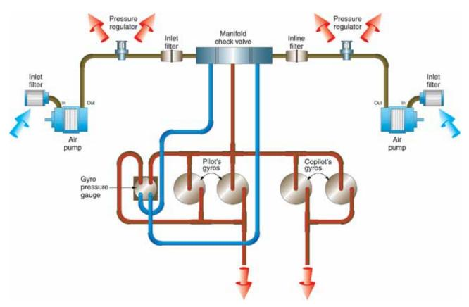
Figure 3-29. Twin-Engine Instrument Pressure System Using a Carbon-Vane Dry-Type Air Pump.
