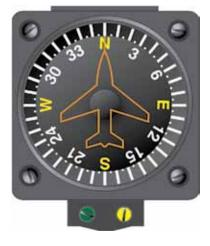
Figure 3-22. Vertical Card Magnetic Compass.
