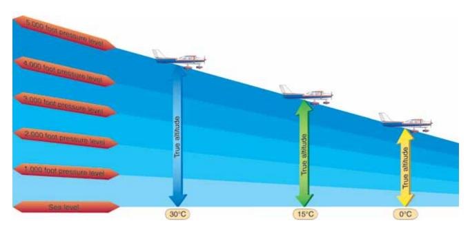
Figure 3-6. The loss of altitude experienced when flying into an area where the air is colder (more dense) than standard.
