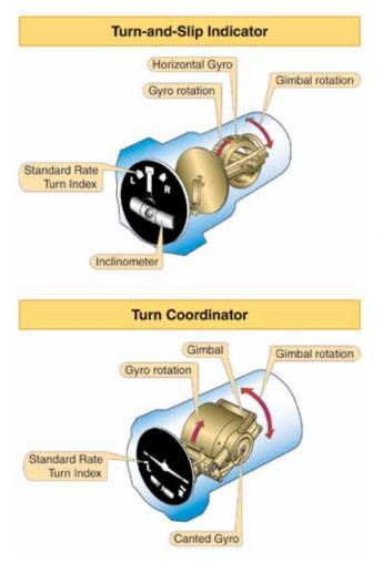
Figure 3-34. The rate gyro in both turn-and-slip indicator and turn coordinator.
