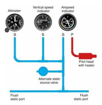
Figure 3-2. A Typical Pitot-Static System.
