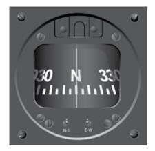
**Figure 3-16.** A Magnetic Compass. The vertical line is called the lubber line.
