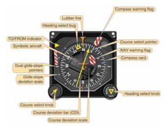
Figure 3-38. Horizontal Situation Indicator (HSI).
