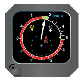
**Figure 3-58.** An example of a resolution advisory being provided the pilot. In this case, the pilot is requested to climb, with 1,750 feet being the appropriate rate of ascent to avoid traffic conflict. This visual indication plus the aural warning provide the pilot with excellent traffic awareness that augments see and avoid practices.
