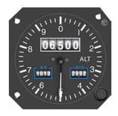
Figure 3-5. Drum-Type Altimeter.
