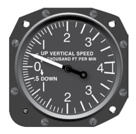
**Figure 3-10.** *Rate of Climb or Descent in Thousands of Feet Per Minute.*
