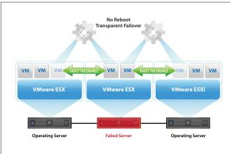
VMware Fault Tolerance enables a transparent failover with no disruption of service in the event of hardware failures
