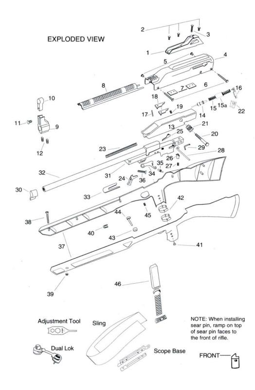
**Safety/Bolt Lock** is located at top of left grip. Sliding safety lever upward, into notch engages safety and places rifle in "SAFE" position.
