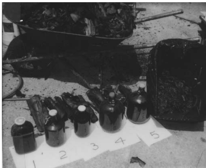
At the end of its August 18, 1993, run Compton's plant had produced the materials pictured here: fifteen to twenty pounds of carbon and three and a half gallons of AAA crude oil. Compton weighed his products on his wife Kathryn's bathroom scale. Image from the Bill Compton Collection.
