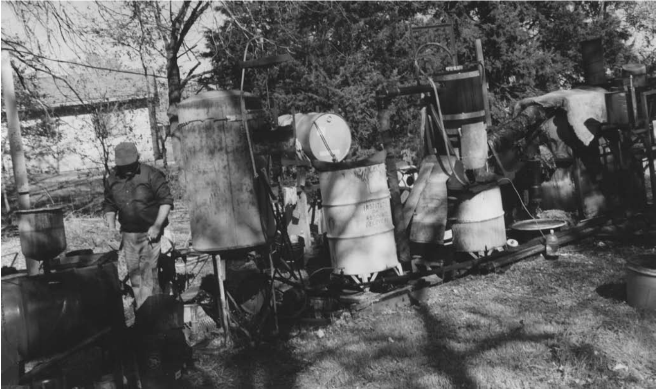
After years of research and planning, Compton decided in 1980 to build his own pyrolysis batch plant, capable of processing one hundred pounds of waste in eighteen hours. He set to work assembling the plant's pieces and parts—many of which were donated by friends—in his front yard. Compton operated his batch plant until August 1984, when he was convinced he had learned all he could from it. In November 1992 Compton constructed a larger pilot plant, which, like the batch plant, was able to process one hundred pounds of material—this time in a ten-hour period. This plant, a section of which is pictured above, operated for a total of 350 hours over a series of years, successfully producing combustible gas, carbon, and oil. Image from the Bill Compton Collection.
