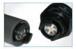
HMAtwo HMAtwo Series is a hermaphroditic fiber optic lens connector that facilitates the interconnection of multiple identical fiber optic cable assemblies (daisy chaining). This eliminates the need for polarizing assemblies and in-line adapters. Lens technology is less vulnerable to contaminants than the traditional physical contact technology. The Connector is available in 1 to 4-way configurations for multi-mode fibers, dual-wavelength 850/1300nm.
