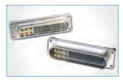
**Ruggedized, Non-Floating Brush Rack and Panel Connector Series** This new connector series utilizes Amphenol's durable and reliable B3 contact system in a rugged, non-floating rack and panel connector. Included in this series are digital and power/digital "hybrid" insert arrangements. The hybrid series utilizes Amphenol's high-performance RADSOK<sup>®</sup> power contacts along with Amphenol's proven B3 contact.
