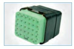
High-Density SIM module The #23 High-Density SIM module is an exclusive innovation of Amphenol's. Based on standard EN4165 SIM Modules, the HD modules have thirty size 23 contacts (BACC47)—an increase of more than 50% over #22 modules. HD SIM Modules are available with or without peripheral overmolded sealing and are fully compatible with all SIM connector series.
