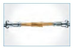
Brush Contact Connectors Multiple strands of high-tensilestrength wire bundled together to form brush-like contacts provides low mating force, extended service life, and stable electrical performance. Brush contacts provides superior electrical characteristics: redundant current paths, minimized constrictive resistance, uniform current densities stable time/ life contact resistance gas tight and electrical contact site integrity, and 20,000 cycles of mating and unmating.
