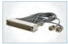
**CMTS Interconnects** Amphenol's CMTS cable harnesses cover either internal or external assemblies for Cable Modem Terminations Systems. The external harnesses typically use bundled 75 0hm cable. Internal cable assemblies typically run no longer than 18," but due to the dense nature of the chassis, special consideration has to be given to the size and flexibility of the cable.
