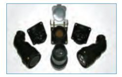
ADG & ADGC Amphenol's ADG Series connectors are used principally in rail mass transit and heavy industry applications. Their main characteristic is the fast and precise coupling of the receptacle and plug connectors. Three bayonet ramps on the receptacle allow for the fast and perfect mating with only a one quarter turn of the coupling nut. They withstand exposure to moisture, oil, and vibration.
