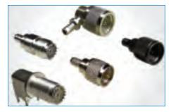
Mini-UHF Mini-UHF is a miniature version of the UHF connectors that were developed for use in the radio industry. Mini-UHF connectors are used as coaxial interconnects in cell phones, automotive systems, and similar applications where size, weight, and cost are critical. Mini-UHF connectors terminate to RG-58, RG-58A, RG-58B, RG-58C, and Belden 9258 cables. Crimptype cable plugs and jacks are available, as well as panel and PCB receptacles.
