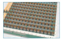
Backplane Assembly Amphenol's design and applications engineering experts apply knowledge gained from thousands of successful backplane designs to your project delivering an integrated backplane system with superior signal channel performance at an optimized cost. We routinely manufacture backplane systems with data rates up to and beyond 20 Gbps with field-proven mechanical reliability.
