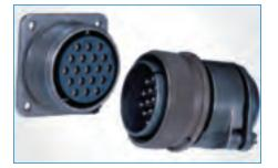
**5015** Amphenol's 5015 Series is a rugged, versatile, and environmental resistant connector with proven electrical capability. 5015 series connectors are medium to heavy-weight cylindrical connectors with 5 shell styles, 19 shell sizes, and 5 service classes. The 5015 offers 286 contact arrangements from 1 to 104 circuits. It is available in solder or crimp contacts, threaded coupling, coaxial and thermocouple contacts, and ROHS compliant versions.
