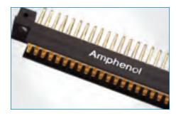
NAFI Interconnect Amphenol's NAFI daughter card and backplane connectors are another board level interconnect solution. They provide a wide range of medium contact density patterns and meet MIL-C-28754 standards. Daughter card termination is through-hole, using nickel/gold solder-plated contacts. The mating interface is a blade contact that can be either parallel or perpendicular to the daughter card.
