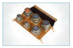
**Rigid Flex Assembly** Amphenol's Rigid Flex capabilities are among the best in the world. Mission-critical applications such as this example are among our standard offerings. The part pictured above is in service in many different fixed-wing fighter aircraft. This part has 16-layers with blind and buried via's assembled with six unique filter connectors on which we perform thermal cycling and level-two testing.
