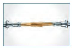
Brush Contacts The brush contact is made up of multiple strands of high-tensile wire that are bundled together. A reduction in mating/un-mating force of 70% to 90% is achieved over conventional contacts. The brush contact has proven low-resistance, durability, and long contact life. Hybrid low-mating force connectors can be designed with combinations of brush and coax, twinax, power contacts, and fiber optic termini.
