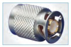
ZMA Connectors and Components The ZMA connector is a bayonet coupling connector. The unique design of this connector provides a high coupling force, which is ideal for extreme vibration applications where insufficient room is available for spring-loaded blindmate panels. This connector is designed with electrical performance of 18 GHz, overlapping PTFE dielectrics, and rugged stainless steel body construction appropriate for military applications.
