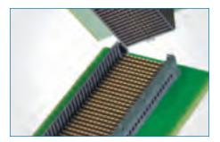
**NeXLev®** Amphenol's NeXLev® high-density parallel board connector is capable of handling data rates up to 12.5 Gbps, providing a robust solution for your increasing bandwidth demands in mezzanine applications. The connector can be routed to support single-ended or differential architectures and offers 20 stacking heights from 10-33mm. NeXLev uniquely applies BGA attachment technology, widely accepted for its high reliability, making it robust both during manufacturing and in the field.
