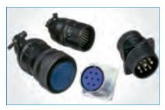
**97** Amphenol's 97 Series is the lowest-cost cylindrical interconnect solution in the proven 5015 family connector style. An extremely versatile connector family, the 97 Series offers six shell options, 128 different contact arrangements, 1 to 52 circuits, one of the largest selections of insert patterns on the connector market, and crimp, solder, thermocouple, and PCB (100 suffix) contacts.
