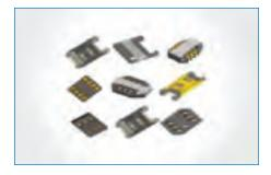
**SIM Card Connectors** Amphenol's extensive range of SIM card connectors is available in three types; wing connectors, bridge block connectors, and SIM block connectors. Available in 6- or 8-contact versions, with and without locating pegs for board stability, all are surface mount types. Many are available with detection switches that allow your device to know if a SIM card is present.
