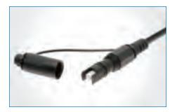
FTTx Cable Assemblies FTTx connectors are used to connect multi-port terminals or fiber terminal closures typically located at the street with Optical Network Terminals (ONTs) via drop cables. This system is installed on the external enclosure surface so that connections can be completed without opening the enclosure, essentially creating a "plug-and-go" connection. Amphenol's optical connector and adapter protects against extreme temperature, moisture, and chemical exposure.
