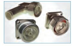
**7/16** The 7/16 series is named for the metric dimensions of the connector interface: 7mm OD of inner contact, 16 mm ID of outer contact. 7/16 connectors are designed for use in communications systems with power levels of 100 watts per channel. These connectors are typically used in antennas, satellite communications, and base stations.
