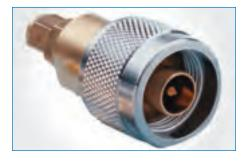
**Precision RF** APC stands for Amphenol Precision Connector and was developed by Amphenol and Hewlett-Packard engineers. The APC is the first instrument-grade coaxial connector series to achieve repeatable TE11 mode resonance-free signal transmission from DC - 50 GHz with a minimum return loss of 26 dB. These 50  $\Omega$  connectors are designed for test and measurement equipment where reliable performance is critical for repeated connect/disconnect cycles.
