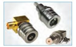
QMA The QMA is a quick-disconnect version of the SMA connector. The electrical performance of the QMA includes low-loss RF performance up to 18 GHz. The QMA connector offers the same high-power handling capability as the SMA connector it is based on. This gives the series significant advantages over other quick-disconnect connectors. Amphenol is a member of the Quick Lock Formula® Alliance.
