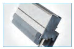
**GbX® Right Angle Male** Amphenol's GbX® Right Angle Male (RAM) enables co-planar board-to-board or board-to-cable high-speed interconnections. Currently available in 2-Pair configurations (27 differential pairs per linear inch), with two different heights — standard RAM and extended RAM. A high-speed differential and L-Series version are also available.
