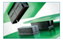
HDM Stacker The HDM Stacker connector optimizes card functionality in a limited space. It can be used in parallel board packaging, mezzanine cards, parallel backplanes, and bridgeboard applications. The connector is available in 72-pin and 144-pin signal modules in soldertail or press-fit configurations. Stacking heights range from 15mm to 32mm.
