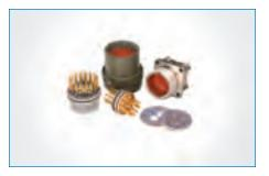
EMI/EMP Filter Products Amphenol's EMI/EMP protection connectors offer the versatility of standard connectors, but with EMI/EMP protection that filters unwanted frequencies for sensitive circuits. By housing EMI/EMP devices internally, you can eliminate costly and bulky exterior discrete protection devices. Available in many sizes, styles, and arrangements, Amphenol filter connectors are inter-mountable and intermateable with standard MIL-spec connectors.
