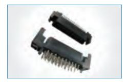
SCA2 (Single Connector Attachment) Amphenol's SCA2 is a type of connector used for internal SCSI cabling systems. "Hot-swapping" allows seamless replacement of failed RAID drives, which greatly simplifies system maintenance procedures. SCA2 features a single plug configuration carrying signal, power, and jumpers together.
