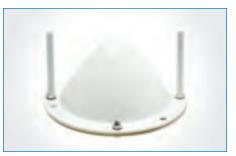
In-Building Antennas Our in-building MPA antennas provide excellent in-building coverage due to effective electrical performance, compact size, and ease of installation. Each antenna is equipped with two reflector pins that can be used to change the azimuth plane from 360° to 180°, 90°, or an elliptical pattern. The MPA is equipped with 30° electrical downtilt to direct the signal toward the floor where coverage is needed.
