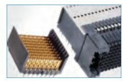
VHDM<sup>®</sup> H-Series VHDM<sup>®</sup> H-Series uses an 0.018" (.045mm) PCB hole for improved routability, which can eliminate costly layers in the printed circuit board, reduce impedance discontinuities, and improve the ability to back-drill, reducing via stub effects. Additional shield-compliant pins on the daughtercard wafer improve signal integrity. VHDM H-Series is backwards compatible and can be designed into the same slot as standard VHDM, enabling data rates up to 6.25 Gbps.
