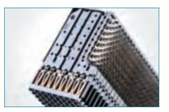
VHDM® The VHDM® connector platform is the industry standard for high-speed backplane applications, with measured performance to 3.125 Gbps and billions of pins installed worldwide. VHDM is available in 6- and 8-Row configurations providing 76 - 101 real signals per linear inch. Stripline shielding allows 100% of the pins to be used for signals.
