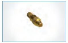
MMCX MMCX (also called MicroMate<sup>™</sup>) is a micro-miniature connector series with a snap-lock mechanism allowing for 360-degree rotation. MMCX connectors conform to the European CECC 22000 specification. The MicroMate Family of products is a 6 GHz 50 Ω interconnect. A range of connectors is available, including surface mount, edge card, and cable connectors. Common applications include broadband, instrumentation, and telecommunications.
