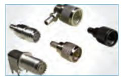
**Mini-UHF** Mini-UHF is a miniature version of the UHF connectors that were developed for use in the radio industry. Mini-UHF connectors are used as coaxial interconnects in cell phones, automotive systems, and similar applications where size, weight, and cost are critical. Mini-UHF connectors terminate to RG-58, RG-58A, RG-58B, RG-58C, and Belden 9258 cables. Crimp-type cable plugs and jacks as well as panel and PCB receptacles are available.
