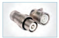
Vortex GT The Vortex GT is a GT shell type connector with reverse bayonet coupling RADSOK<sup>®</sup> technology, designed specifically for delivering high-power from source to load. The plug contact is an 18mm crimp type RADSOK<sup>®</sup> socket combined with an 8mm RADSOK<sup>®</sup> pin. The receptacle contact is an 8mm screw type RADSOK<sup>®</sup> pin combined with an 8mm RADSOK<sup>®</sup> socket. Uses include electrical generators, fuel cells, load banks, and charging systems.
