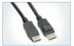
DisplayPort Connectors Amphenol now creates DisplayPort connectors and cable assemblies. DisplayPort is a new digital display interface standard put forth by the Video Electronics Standards Association (VESA). It is a next generation digital interface that is designed to replace LVDS, DVI, and eventually VGA. It covers provisions for high-definition digital audio-video and graphics streaming via the interface through the same cable.
