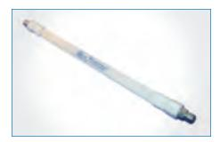
**Window Jumper** Amphenol's Window Jumper is a 12" flat cable assembly designed to allow the easy installation of cable or satellite television or Internet service without having to drill through walls. The cable assembly is extremely durable and was designed to withstand at least 50,000 window opening/ closing cycles. It is also resistant to temperature fluctuations from -40° to 80° C and salt spray.
