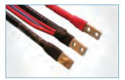
POWERLUG Amphenol's POWERLUG cable termination is formed from contiguous copper stranding, eliminating the crimp joint of standard ring terminals. This significantly increases cable termination reliability while reducing the MV drop inherent within a crimp joint. Closer spacing is allowed as the joint diameter does not exceed the diameter of the terminated cable. Available in standard or custom POWERLUG configurations.
