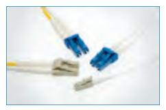
LC Cable Assemblies Amphenol's fiber optic LC small form factor connector cable assemblies provide high-density connections for a variety of telecommunications applications. Amphenol utilizes TIA 604-10, IEC 61754-20 compliant one-piece body connectors for assemblies. Connectors are available in 900um, 2mm, or 3mm, and simplex or duplex. Multiple cable constructions are also available.
