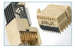
AirMax VS® The AirMax VS® connector utilizes edge-coupling technology to improve electrical impedance control with optimized stagger to minimize signal crosstalk. This innovative combination delivers a cost-effective interconnect for multi-gigabits/s applications. To leapfrog traditional complex Stripline designs, the AirMax VS solution utilizes "Virtual Shields," which eliminate costly metal interleaves between columns. \*\*AirMax VS is a registered trademark of FCI.
