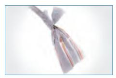
Twist 'n' Flat Amphenol's .025 pitch Twist 'n' Flat cable is designed for internal interconnection of parallel SCSI drives. Amphenol has long been the industry standard for precision mass termination flat cables. Cables are typically 68 conductor 30 AWG, with either PVC or TPE dielectrics, depending on customer impedance requirements.
