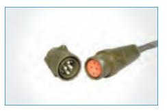
MIL-Power Heavy-Duty Circular Connectors Originally designed for use by the military, Amphenol's heavy-duty circular connectors have become widely used in aerospace, ground support, and shipboard applications. Some features include quick positive coupling, waterproof-IP67 rated, no lockwiring required, high shock and vibration capabilities, and are available in both crimp and solder terminations.
