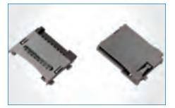
Memory Card Sockets Amphenol offers a full range of flash memory connectors (including SD, Mini-SD, Micro-SD, xD, CF1 & 2) with numerous features such as low-profile design, normal or reverse mounting, manual or push-push insert style, and a locking feature to prevent the card from dropping out. Available in SMT, straddle mount, or through-hole termination.
