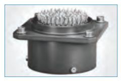
Amphemol Press Fit Connectors Amphenol manufactures a complete series of MIL-DTL-38999 Series I, II, and III connectors with Press Fit compliant pin contacts for solderless mounting on printed circuit boards. Both pin and socket contacts are available in any MIL-DTL-38999 series I, II, or III insert pattern having contact size 16, 20, or 22D. Press Fit connectors allow for simplified board assembly while eliminating problems inherent in soldering connectors to boards.
