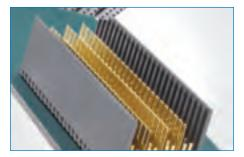
**GbX®** Amphenol's GbX® connector is a high-density optimized differential connector offering a choice of density configurations. GbX provides increased density, exceptional impedance matching, and low crosstalk. GbX delivers data rates of 5 Gbps and is ideal for 4 x 3.125 XAUI links. The GbX connector provides up to 69 pairs per linear inch (5-Pair configuration) with a choice of configurations (2-, 3-, 4-, and 5-Pair) for higher application flexibility.
