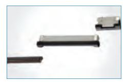
**FPC** Amphenol Flexprint connectors (C007 series) accommodate 0.3 mm thick flexprint cable with different contact configurations and pitch sizes. The double-sided, pre-stressed contact shape guarantees secure contact between the flexprint circuit and the connector, and allows insertion of the flexprint cable in either upward or downward direction.
