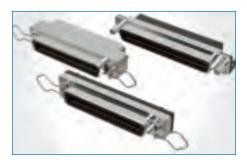
Filtered Connectors Amphenol's FCC57 series of filtered micro-ribbon connectors provides a very cost-effective solution to combat EMI. The family of connectors is the telephone industry's standard for multiple line connections. Available in 36, 50, and 64 sizes with a variety of termination styles, including: male/female, right angle PCB, vertical, press-fit, and solder cup.
