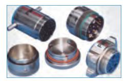
83538 Weapons Release The 83538 Weapons Release Connector was designed for use on aircraft that carry rail launch missiles such as AMRAAM. With buffer plug and missile receptacles, the connector is designed for blindmating of stores on rail launch applications. Used on F-18, B- 52, B-2, and SRAM II programs. The 83538 meets the applicable specifications of MIL-STD-1760 Stores Management.
