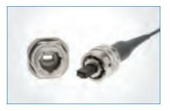
**PT/MPO Cable Assemblies** The Industrial PT/MPO leverages the proven MIL-Spec 26482 connector system to provide an environmental seal and mechanical protection for an MPO-style connector. The metal bayonet connector system is quick to deploy, requiring only ¼ turn. The PT/MPO connectors are exceptionally well suited for WiMax, wireless, and base station applications.
