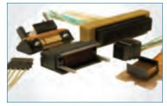
VHDM<sup>®</sup> Cable Assemblies Amphenol's VHDM<sup>®</sup> Cable and Flex Assemblies are the cable solution complement to Amphenol's broad VHDM backplane product family. The VHDM backplane system is a 3.125 Gb/second capable connector system on a 2 mm x 2.25 mm grid. Crosstalk is held to less than 5% through the connector.
