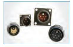
**38999 PowerSafe** Amphenol's PowerSafe connector is directly derived from the MIL-DTL-38999 Series III. The connector series can accommodate power platforms from 13 to 100A per contact and is equipped with "First Mate Last Break" contacts connected to the shell. The grounded FMLB contact will stay in the right position even if the insulator of the connector is destroyed by fire.
