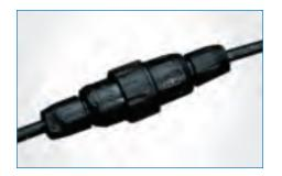
Barracuda The Barracuda range of environmental IP68 sealed connectors is specifically designed for harsh applications where water, dust, oil, or spray is present. These molded connectors are interchangeable with the equivalent Bulgin standard Buccaneer range of connectors, which feature enhanced ergonomics and ruggedized moldings. The Barracuda bodies are molded from glass filled nylon and all have the same outside diameter of 38mm at the largest point.
