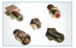
**Type F** Amphenol knows that low-performance F receptacles could not be used in high-speed cable modems and customer interface units (CIUs). The industry has challenged connector manufacturers to develop high-performance connectors featuring -30 dB return loss at 1 Ghz – Amphenol has met this challenge. Our high-performance F-connectors comply with a 3/8-32 thread specification. Primary applications are for cable television (CATV), set-top boxes, and cable modems.
