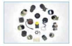
**62IN** 62IN series connectors are general-purpose, environment-resistant, miniature circular connectors with three-point bayonet coupling and five-key polarization. Designed to meet the requirements of MIL-C-26482 Series I solder type, these connectors are widely used in military and industrial applications.
