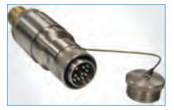
**Optron Hybrid Connectors** Amphenol's Optron connectors are a complete line of circular hybrid connectors designed and qualified to MIL-PRF-28876, Rev. E. They are precision machined and designed to provide superior optical performance in extreme environmental conditions. The Quickloc backshell also allows easy access to maintain or reconfigure termini without altering the captivated aramid fiber.
