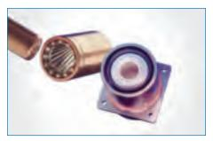
**RADSOK®** Amphenol can upgrade many core connectors and offer custom connector solutions by adding our patented RADSOK® contact. RADSOK® is a RADial SOcKet that was developed from a flat, stamped grid, twisted into a hyperbolic geometry to form a socket contact with unique characteristics. The hyperbolic grid maintains more current by having a greater conductive surface area. Unique features of RADSOK include high reliability, lowvoltage drop, high cycle durability and low insertion force.
