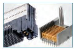
VHDM-HSD<sup>™</sup> The VHDM-HSD<sup>™</sup> connector is a shielded, high-density, high-speed press-fit connector system optimized for differential pair architectures. A modular design allows all the features and functionality required in a system to be integrated in a single robust connector. VHDM-HSD delivers data rates up to 5 Gbps, scalable to 10 Gbps with backwardscompatible eHSD<sup>®</sup> connector. Available in 5-, 6-, and 8-Row versions.
