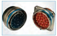
MIL-DTL-38999 Series I LJT, Series II JT The LJT Series I has a longer shell to provide 100% scoop-proof protection for recessed pins. The JT Series II connector has a low-profile shell for maximum weight and space savings. Both series incorporate three point bayonet mating/unmating and five-key/ keyway polarization. The LJT and the JT series feature crimp termination and rear-release contacts.
