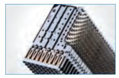
VHDM<sup>®</sup> The VHDM<sup>®</sup> connector platform is the industry standard for high-speed backplane applications, with measured performance to 3.125 Gbps and billions of pins installed worldwide. VHDM is available in 6 and 8-row configurations providing 76 - 101 real signals per linear inch. Stripline shielding allows 100% of the pins to be used for signals.
