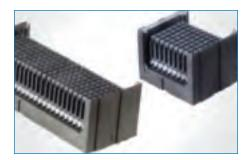
VHDM<sup>®</sup> Stacker Amphenol's VHDM<sup>®</sup> Stacker allows the design of parallel board-to-board connections with the high-speed, high-density performance of standard VHDM. The connector utilizes press-fit compliant pins which can be routed singleended or differentially. Zero and 15 column modules are available with stacking heights from 18mm and up. The VHDM Stacker delivers data rates of 3.125 Gbps with 76-101 real signals per linear inch.
