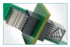
**Crossbow™** The Crossbow<sup>™</sup> connector system is the first differential connector truly optimized for orthogonal midplane applications. Crossbow is designed so the differential pairs on each side of the midplane share vias, allowing designers to take full advantage of the benefits associated with orthogonal midplane architectures. With 20+ Gbps performance, Crossbow meets the IEEE 802.3ap v3.2 10GBASE-KR standard with margin, ensuring compliance with future 10 Gbps specifications.
