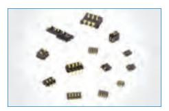
Battery Connectors Amphenol's comprehensive offering of battery connectors for mobile phones come in single and multicontact versions with straight and right angle mountings. They are available in a variety of pitches and heights to meet different phone and battery pad requirements. They feature stamp and form beryllium contacts with additional solder tags for high reliability and conductivity.
