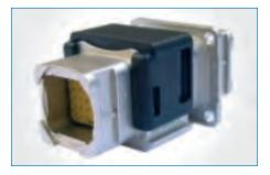
SIM2B 20 Monomodule Connectors These rectangular connectors are modular, multi-contact, multi-functional mono-module connectors, for in-flight entertainment and cabin systems interconnects. These light-weight composite products are available in metallic or non-metallic versions. They present a very compact design with a push pull locking system for blindmating and 4 keying positions.
