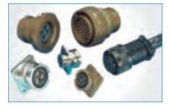
ACA-B The ACA-B is designed for commercial and industrial environments requiring a rugged bayonet style connector for heavy duty power and signal applications. A comprehensive selection of insert arrangements and accessory hardware configurations is featured to accommodate heavy-duty commercial wire and cable. ACA-B is manufactured in accordance with MIL-C-5015 and VG95234. The insulators are made of high-quality polychloroprene material and withstand temperatures of -55° C to +125° C.
