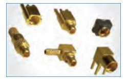
**MMCX** MMCX (also called MicroMate<sup>M</sup>) is a micro-miniature connector series with a snap-lock mechanism allowing for 360-degree rotation. MMCX connectors conform to the European CECC 22000 specification. The MicroMate family of products is a 6 GHz 50  $\Omega$  interconnect. A range of connectors are available, including surface mount, edge card, and cable connectors. Common applications include broadband, instrumentation, and telecommunications.
