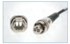
PT/LC Cable Assemblies The Industrial PT/LC leverages the proven MIL-Spec 26482 connector system to provide an environmental seal and mechanical protection for a duplex LC connector. The PT/LC connectors are capable of performing in the toughest environments, making them exceptionally suited for WiMax, wireless, and base station applications. Multiple receptacle configurations and cable types are available.
