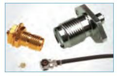
AMC Amphenol's 50  $\Omega$  AMC cable assemblies are ideal for space-constrained board-to-board connections in small devices. Their snap-on interface performs superbly under shock and vibration conditions, making them ideal for wireless handheld devices. The AMC series has a low profile (2.5 mm off the board) and offers an extremely small board footprint (3 mm x 3 mm). This series is compatible with the U.FL interface.
