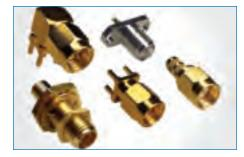
SMA SMA is an acronym for sub-miniature version A and was developed in the 1960s. It uses a threaded interface. 50  $\Omega$  SMA connectors are semi-precision, subminiature units that provide excellent electrical performance from DC to 18 GHz. These high-performance connectors are compact in size and mechanically have outstanding durability. SMA connectors are used in phase array radar, test equipment, ILS landing systems, and other instrumentation.
