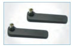
PC Card Antennas Amphenol's series of miniature data card antennas for 2.5 and 3G applications provide the performance to power high-speed mobile internet connectivity. With volumes less than 1.5cc and a customizable geometry these multiband antennas are easily integrated into miniature data cards. The data card antennas can be combined with diversity antennas in the card to further improve the reception.
