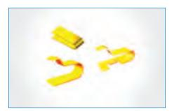
Spring Clips Amphenol's spring clips can be used in the following applications: antennas, metal housing connections, grounding connections, shielding connections, ESD & EMC connections, and LSD connectors, to name a few. They can incorporate a deflection stop to avoid permanent deformation of the clip. Scalable height for platform use. SMT solderable. Packed in tape & reel. Pick & place capable.
