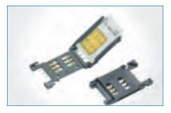
SIMLOCK® Amphenol's SIMLOCK® was designed for SIM/SAM card applications. The SIMLOCK features dimensions only slightly larger than the SIM card. The closed system with integrated card guidance assures reliable contacting of the SIM card, meeting critical card tolerances as per GSM 11.11. The polarization notch does not allow incorrect card positioning. Suitable for automatic assembly processes: pick & place, tape & reel packaging, and SMT solderable.
