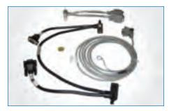
Battery Harness These cables form an alarm harness in an Uninterruptible Power Supply system. The specially designed D-sub assemblies are tested water-tight at a depth of 3 meters (10 feet). This ensures reliable signal interconnect performance under the severe conditions typically encountered in outside cabinets. Individual assemblies permit substantial variation in length, configuration, and form factor for completed harnesses.
