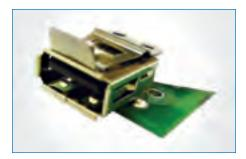
**USB with Positive Locking: LUSB Series** Amphenol's USB, Series A with a unique latching mechanism has been developed to address major concerns of unintentional interruption of data transmission. This patented, unique latching mechanism must be intentionally raised in order to remove the plug. An accidental pull on the cable up to 22 lbs force will not separate the connectors.
