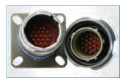
**38999 High-Density** Amphenol has developed a full range of high-density inserts to fit in MIL-DTL-38999 shells or derived products. These inserts allow a contact density increase of 45% versus a standard MIL-DTL-38999 connector equipped with size 22D contacts. These high-density inserts can accept MIL-Spec crimp contacts, as well as contacts with PC tails. These inserts are compatible with all the derived product ranges.
