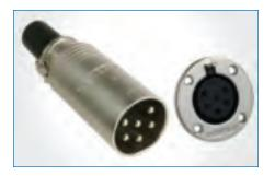
**EP Connector** The EP/AP Series offers consistently superior power-handling capabilities. The EP series incorporates a rugged zinc die-cast shell to give maximum durability when used in demanding situations. The AP Series Shell is manufactured from tough, durable thermoplastic and is ideal for fixed indoor installations. Both the EP and the AP series utilize the same contact and insulator components.
