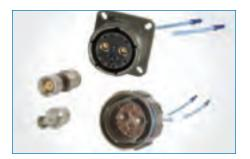
HF38999 High-Frequency Contacts Amphenol now offers DC to 40 GHz size 8 coaxial contacts for the D38999 housing and standard inserts. These contacts can be terminated to many cable types depending on the application. By using standard interfaces that are based on MIL-STD-348 and can be installed in any D38999 size 8 insert, Amphenol has transformed the circular connector industry.
