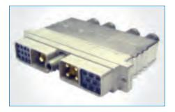
**SIM Connectors** Amphenol's SIM connectors are modular, multi-contact, multi-functional rectangular connectors. They come in metallic or composite versions, shielded or not, and are qualified according to the EN4165 spec. SIM connectors can be a standard or flange-mount receptacle that can be assembled side by side on a panel with standard or rack and panel plugs as well as other options.
