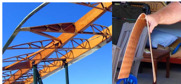
Handmade ribs by Kip, hand bent veneer for the wings by Brent.
