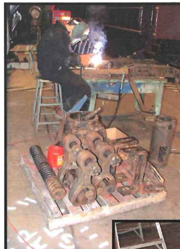
610: 0-8-0? – Number 610 had several repairs completed before entering her 21st year of service at TVRM. Among other things, the lead truck was removed and the frame renewed. At right shows the wheel-less front end over our drop pit and below are the springs and rigging components for the lead truck as Shop Foreman George Walker welds on the frame.
