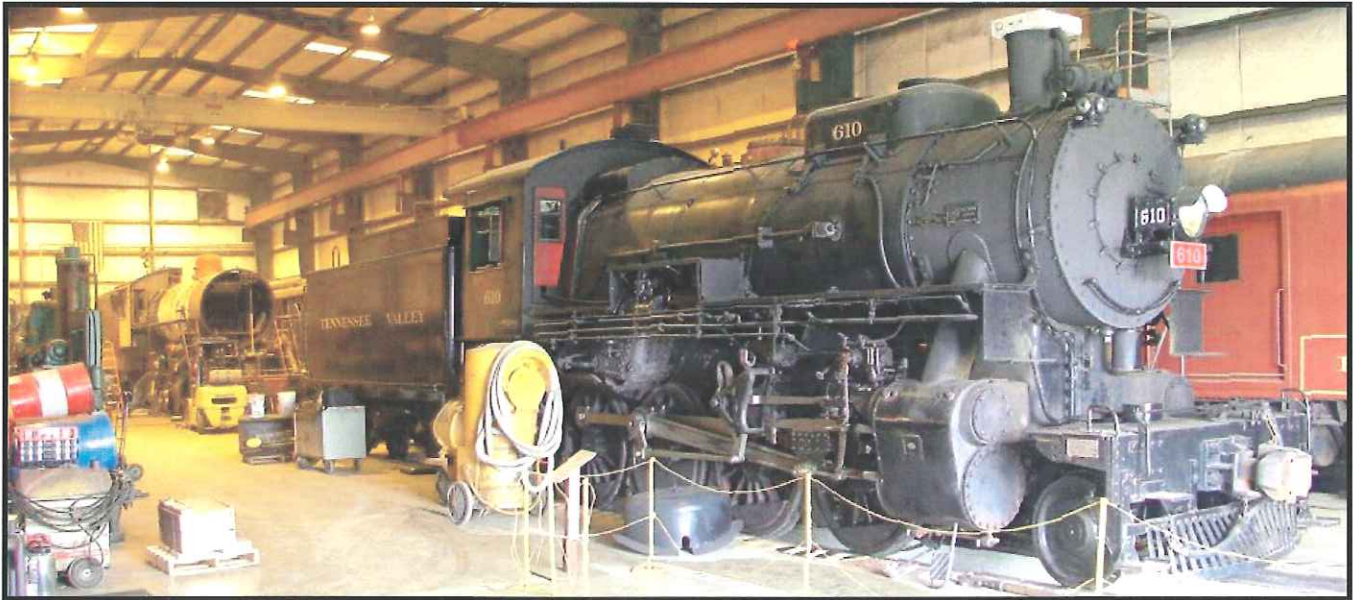
BACK TOGETHER – Seen inside Soule Shops at the end of February, Number 610 is being readied for service. Notice its steam dome cover adjacent to the drive wheels, and Locomotive #630 in the background.
