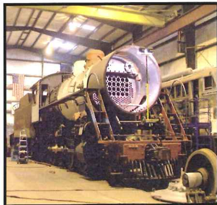
FRONT SHOT – At left is a view of #630 from mid-January. A spotlight was in place which highlights the front fluesheet and the superheater header. As months went on, more components were replaced such as the smokestack.
