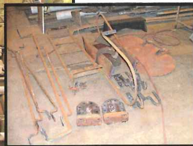
As previously reported, #630's tank was severely deteriorated (as was #4501's old one) and using #4501's longer tender frame as a base for the new tank will allow additional coal and water capacity.
