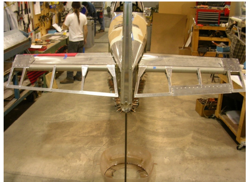
Horizontals built & elevators installed
