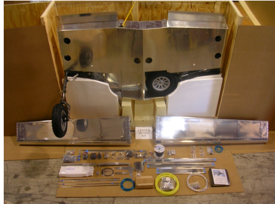
This photo shows everything that is included in the Center Section Kit.
