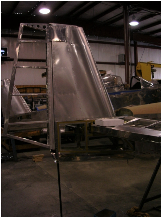
Vertical Stabilizer & rudder installed straight from factory.
