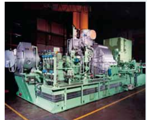
The turbogenerator set for M/S Gudrun Mærsk incorporates an exhaust-gas power turbine (left side), the generator (right side) and a steam turbine (centre).
