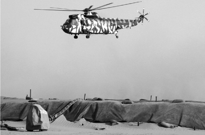
The provision of fuel in the field – a Royal Navy Sea King and a desert pillow tank farm.
