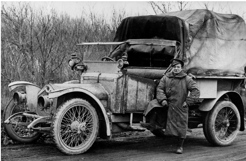
Representative of the kinds of vehicles used by the RFC/RAF to move supplies around – a 25hp Crossley tender.
