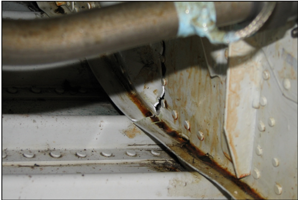
Figure 4: Example of rear pressure bulkhead damage
