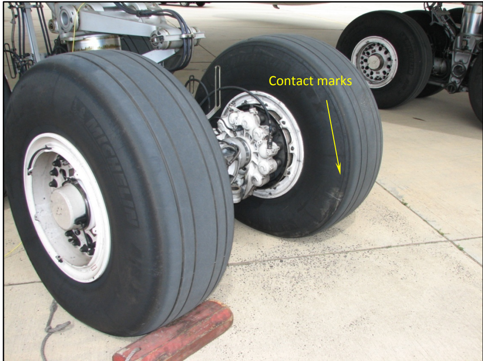
Figure 7: Contact mark on left main landing gear, inboard rear tyre
