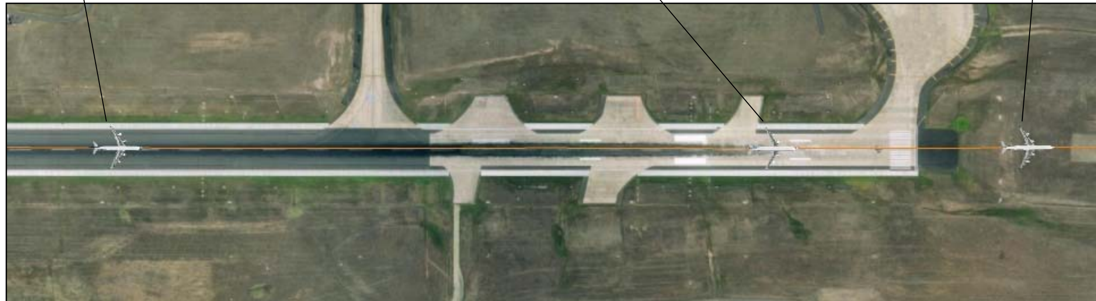
Figure B4: Graphical representation of DAR data showing position of aircraft at a computed airspeed corresponding to V1 used by the crew, initial tail contact with ground, and final tail ground contact witness mark.
