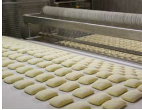
A hanging wire-mesh belt ensures that the dough pieces are accurately handed over to the mounting conveyor belt by applying soft pressure from above.
