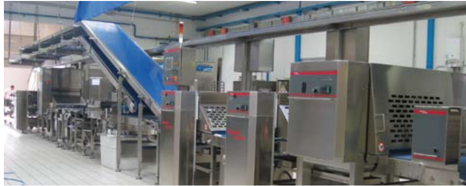
The new speciality bread line is installed in the competence centre of Rondo Doge in Schio.
