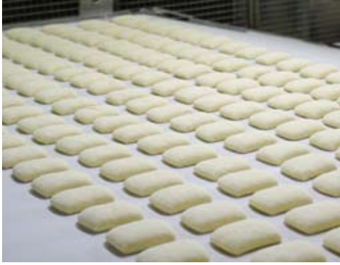
In Holstebro, Denmark, Lantmännen produces on one line partly-baked bakery products of very soft dough with high water absorption and long dough rest.
