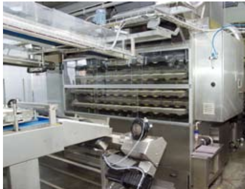
After a short pre-proofing, the round dough pieces reach the long moulders via conveyor belts.
