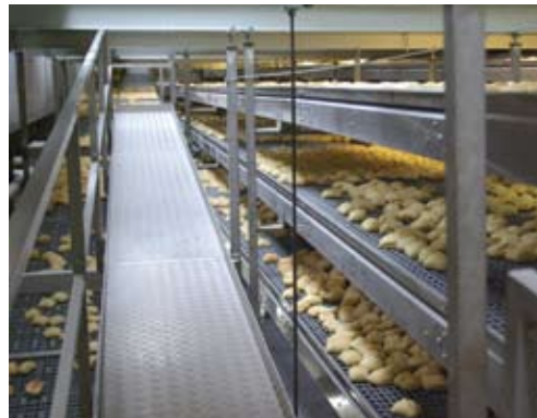
The bread rolls slowly cool down to ambient temperature on the transport belts.
