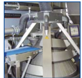
The conical round moulder is equipped with fan nozzles. The tempered air blows moisture off the dough surface and thus prevents that the dough sticks to the moulding cone which works like the other components of the line also consequently without separating agent.
