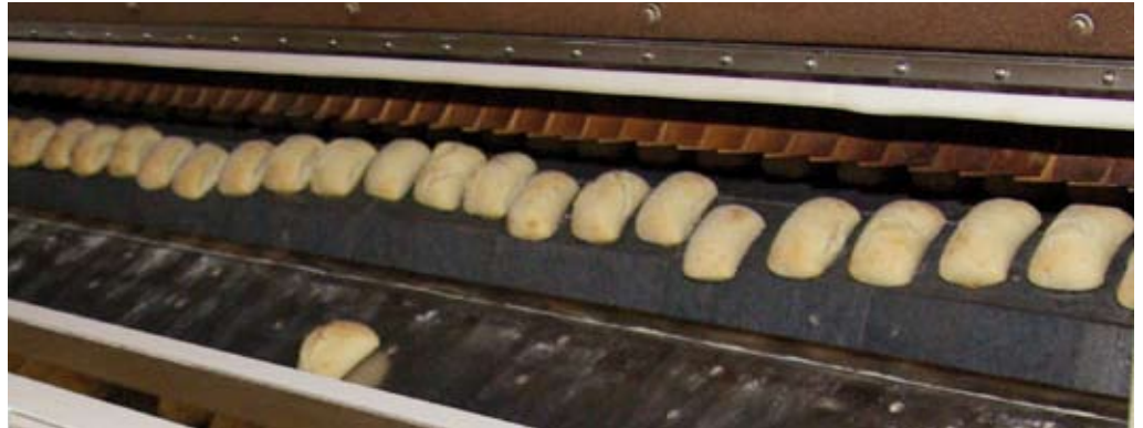
On this picture the bigger diameter of the stone plate belt at the diversion is clearly visible. The bakery products slide from the belt onto the unloader.
