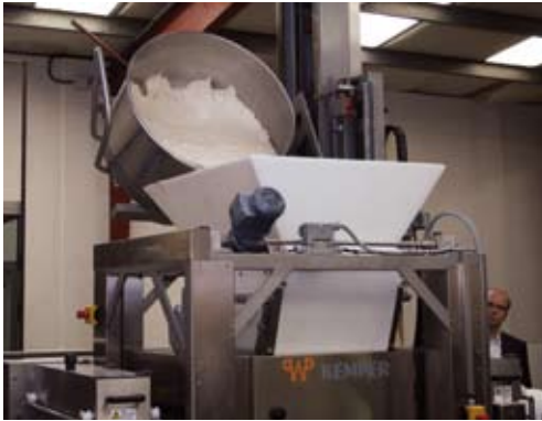
Instead of a batch-wise dough infeed by means of a lift tipper, the line can also be continuously fed with dough.
