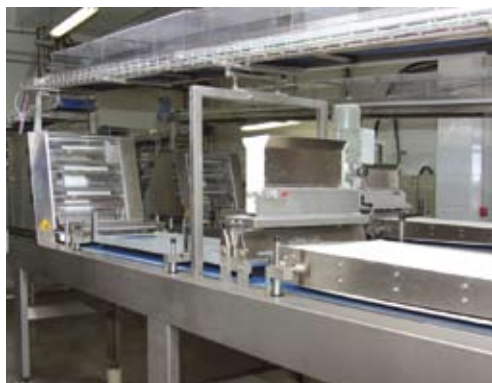
In the long moulder, the dough pieces are reduced, coiled up and gently brought into the desired shape over a very long moulding distance.
