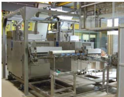
Different weight ranges: A particularity of the line are the two dough dividers of the type Industrie Rex which can be moved on rails under a dough hopper which is mounted fix on an underframe.
