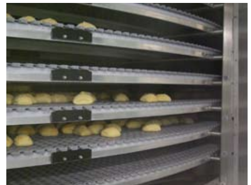
Finally, the bakery products are frozen in the shock freezer and then packed.
