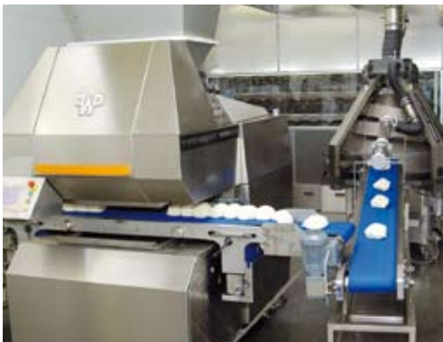
In every line a modified dough divider V 700B by W&P Haton is used without hybrid piston but with a reduced oil consumption.
