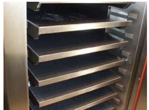
A wagon oven with stone plates on the radiators, on which it is possible to bake directly.
