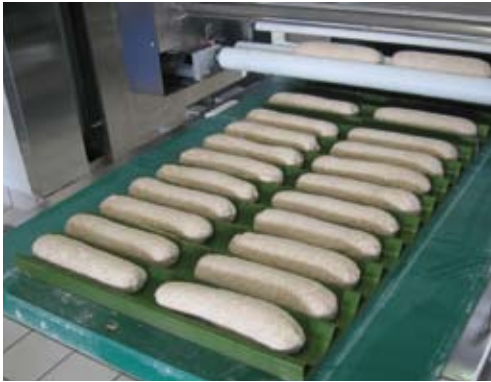
The station to deposit the long moulded breads onto baking trays.
