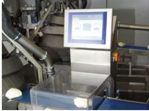
Lower than one percent: Weight exactness is important in Russia. The indicated weights per piece on the check-weigher have all been below one percent during our visit.
