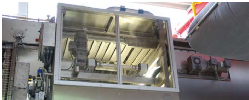
Turned upside down: brushes clean the carriers from below. Moreover they are disinfected by means of IR-radiation.
