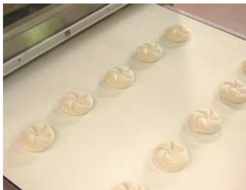
Transfer of the dough pieces into the final proof-er. As an alternative, they could also be trans-ferred as unproofed dough pieces directly into the spiral freezer.
