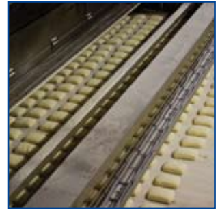
The infeed of the stone plate belt is particularly challenging, as the thicker stone plates and the suspension increase the diameter at the diversion of the belt at the infeed and at the exit of the oven.
