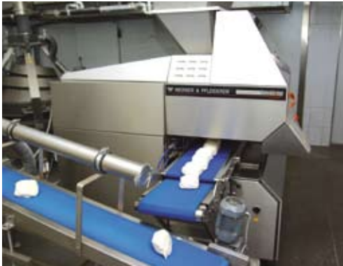
Nozzles in the pipe above the belt blow tempered air over the moist dough surface.
