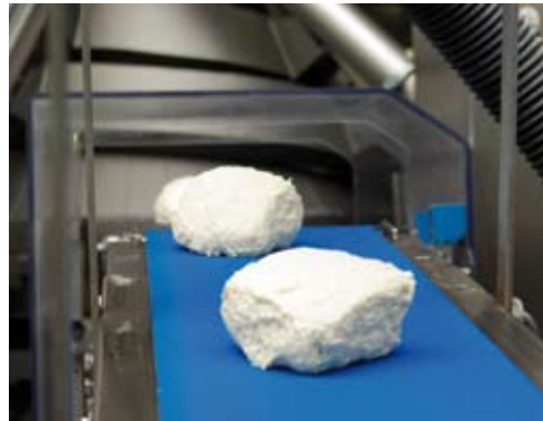
The V700B cuts 6,000 pieces per hour, which are distributed via conveyor belts into two conical round moulders.
