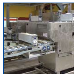
The hopper is mounted fix on a frame above the dough divider. Depending on the product weight, the first or the second dough divider is used.
