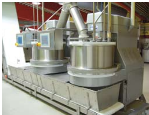
Two Diosna kneaders feed the König line. The dough is transported through the bottom discharge of the kneaders via a conveyor belt into the supply hopper above the dough divider.
