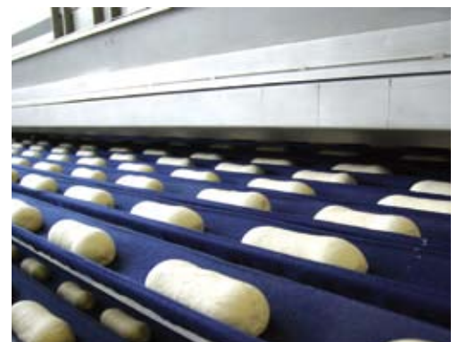
During the transfer into the proofer, there is no cycle, but a continuous movement of the carriers running synchronously with the belt speed of the oven.
