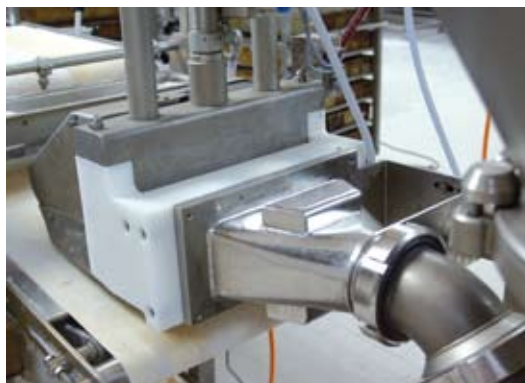
The dough divider extrudes a dough strand which is portioned in the attachment by means of a guillotine. To achieve a perfect cut, the double screws in the divider stop during the cutting process.
