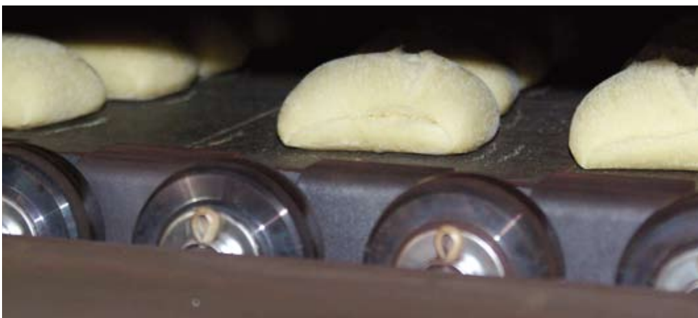
Bakery products on the stone plate belt. At first, the heat application is quick and direct, but is then buffered by the stone.
