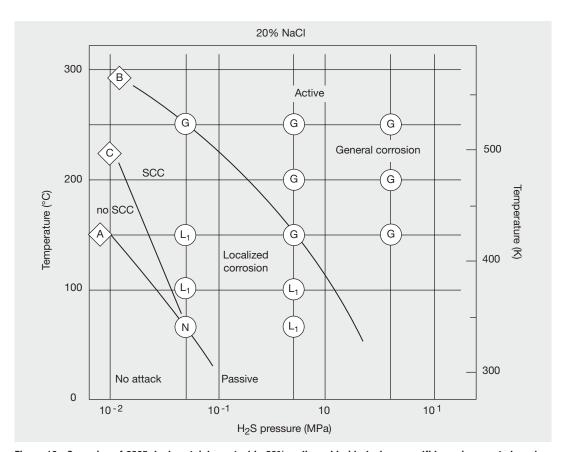
Figure 10: Corrosion of 2205 duplex stainless steel in 20% sodium chloride-hydrogen sulfide environments based on electrochemical prediction and experimental results.
