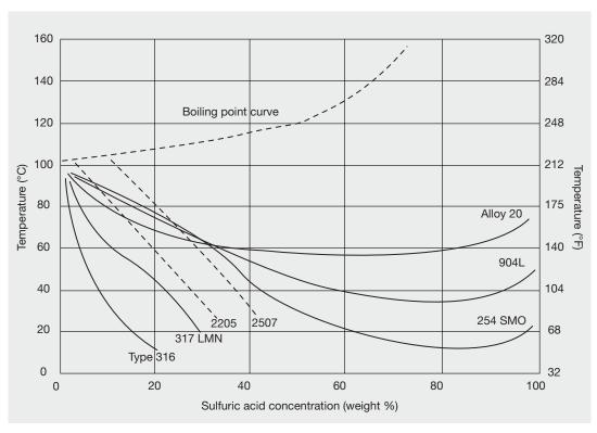
Figure 6: Corrosion in non-aerated sulfuric acid, 0.1 mm/yr (0.004 inch/yr) isocorrosion diagram (laboratory tests using reagent grade sulfuric acid). (Source: Producer data sheets, 254 SMO is a trademark of Outokumpu)
