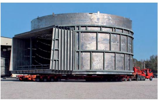
Flue gas desulfurization unit fabricated using 2205 stainless steel (Source: ArcelorMittal)
