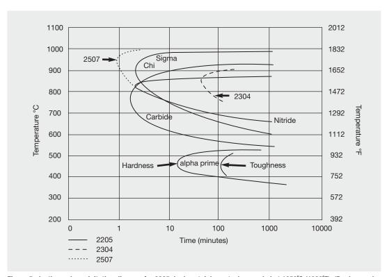
Figure 5: Isothermal precipitation diagram for 2205 duplex stainless steel, annealed at  $1050^{\circ}$ C ( $1920^{\circ}$ F). (Duplex grades 2304 and 2507 are shown for comparison)
