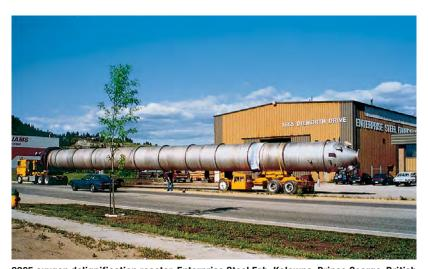
2205 oxygen delignification reactor, Enterprise Steel Fab, Kalowna, Prince George, British Columbia, Canada (Source: Outokumpu)
