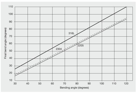
Figure 12. Comparison of springback of duplex stainless steels and type 316L for 2 mm (0.08 inch) thick sheet (Source: Outokumpu)
