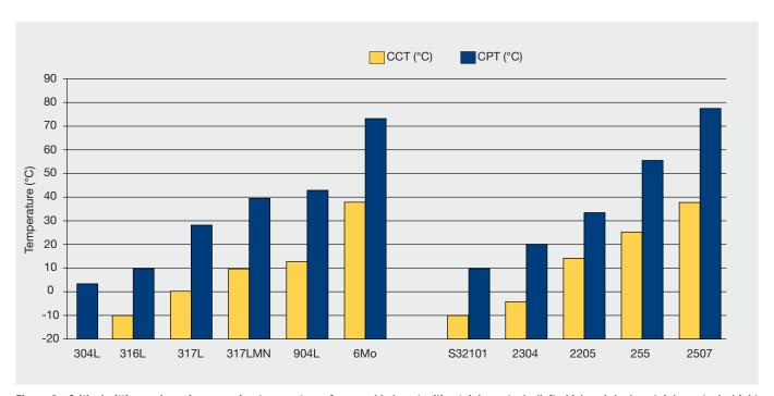
Figure 8: Critical pitting and crevice corrosion temperatures for unwelded austenitic stainless steels (left side) and duplex stainless steels (right side) in the solution annealed condition (evaluated in 6% ferric chloride by ASTM G 48)
