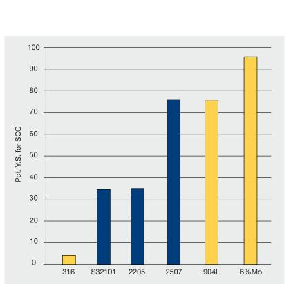
Figure 9: Stress corrosion cracking resistance of mill annealed austenitic and duplex stainless steels in the drop evaporation test with sodium chloride solutions at 120°C (248°F) (stress that caused cracking shown as a percentage of yield strength) (Source: Outokumpu).
