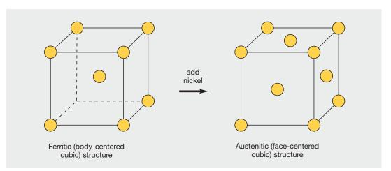
Figure 1: By adding nickel, the crystallographic structure changes from body-centered cubic (little or no nickel) to face-centered cubic (at least 6% nickel – 300 series). The duplex stainless steels, with their intermediate nickel content, have a microstructure in which some grains are ferritic and some are austenitic, ideally, about equal amounts of each (Figure 2).
