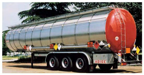
Lean duplex stainless steel asphalt hauling tanker (Source: Outokumpu)
