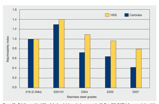
Figure 15. Relative machinability of duplex stainless steels compared with Type 316 (2.5Mo) for cemented carbide tooling and for high speed steel tooling (Source: Outokumpu)
