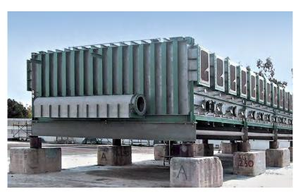
Multi stage flash seawater desalination unit constructed of S32101 and S32205 duplex stainless steels (Source: Outokumpu)
