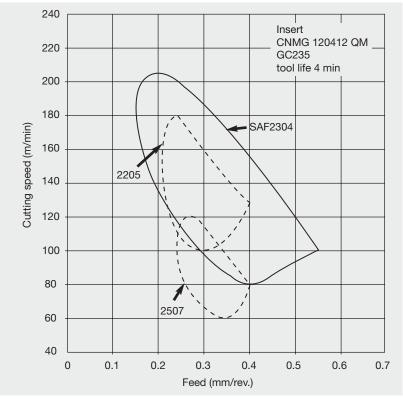
Figure 16: Comparison of machining parameters for turning duplex stainless steels with a cemented carbide insert with a tool life of four minutes (Source: Sandvik)
