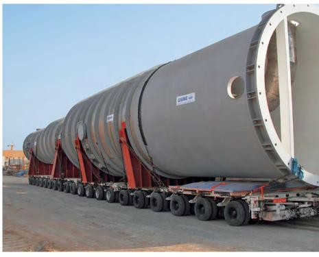
2507 stainless steel falling film evaporator (Source: Gary Carinci, TMR Stainless)
