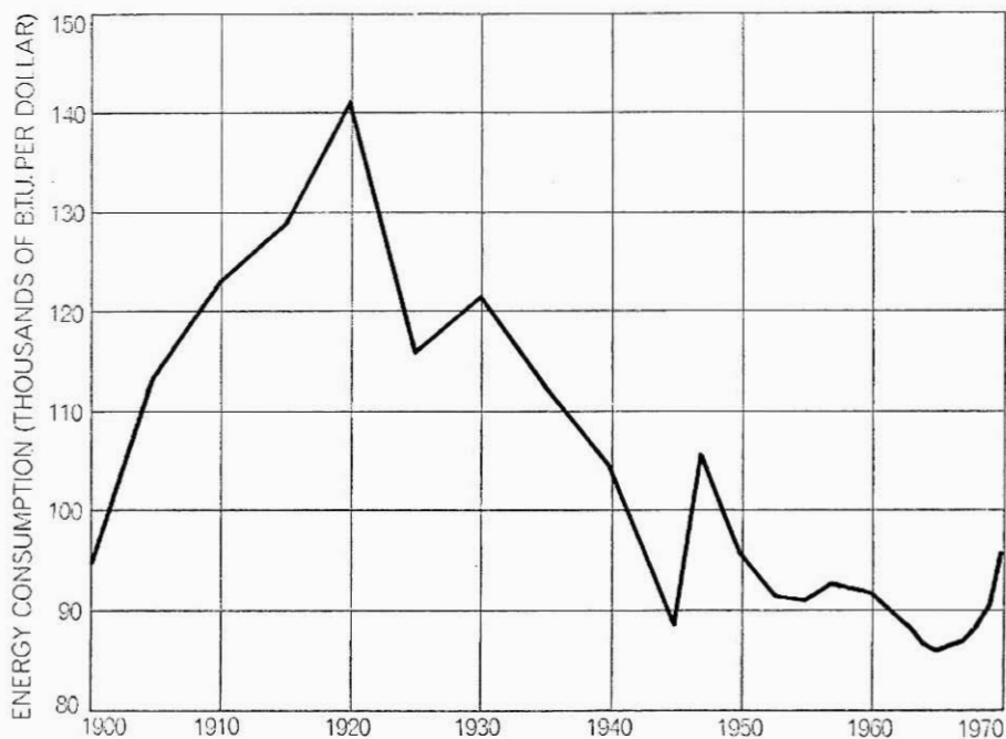
RATIO OF ENERGY CONSUMPTION to gross national product has varied over the years. It tends to be low when the G.N.P. is large and energy is being used efficiently, as was the case during World War II. The ratio has been rising steadily since 1965. Reasons include the increase in the use of air conditioning and the lack of advance in generating efficiency.
