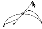
As you drag the BCP left or right, the other BCP moves along with it.
