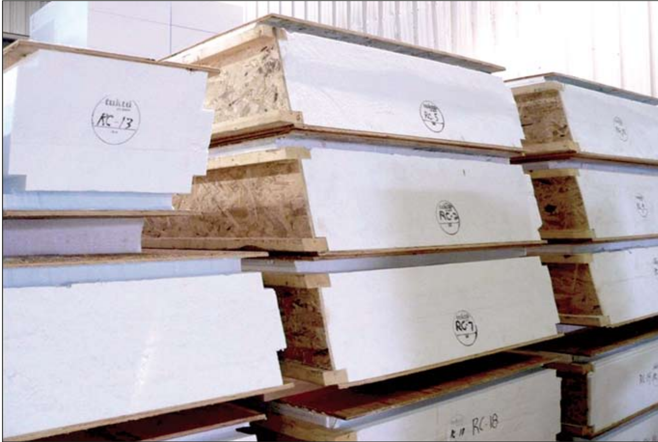
Out of the 285 public housing units planned for construction, roughly 140 will be built using energy efficient structural insulated panels, seen here.
