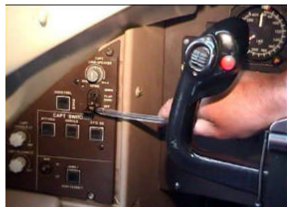
Figure 6 : Three-position GPWS switch in OFF position
