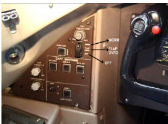
Figure 5 : Three-position GPWS switch in NORMAL position
