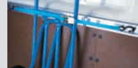
Side cargo storage rail Allows loads to be easily and securely lashed. (Option - load strap not supplied. Shown with load compartment trim board)
