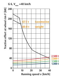
Starting effort acc. to Curtius and Kniffler, train resistance on level track calculated using formula for complete trains of Fal-waggons acc. to DB
