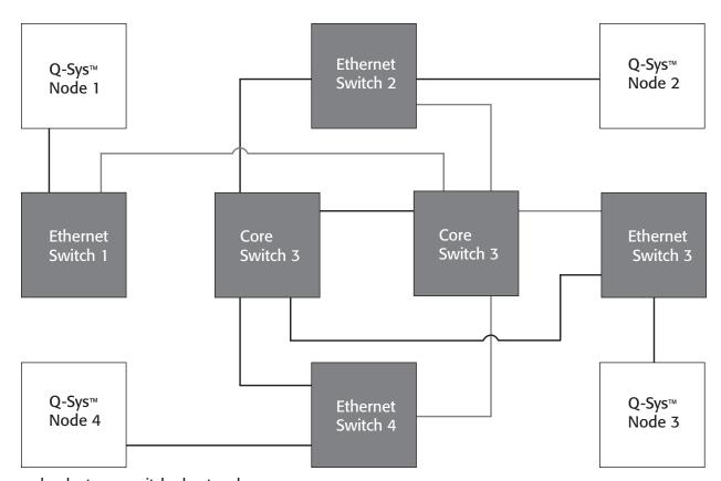
4-hop redundant core switched network
