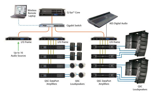
The Core's connection to the rest of the system is primarily through the Q-LAN network. Each Core has four gigabit Ethernet connections: two for fault-tolerant Q-LAN and another two for running control communication though connections physically separate from Q-LAN if desired. Q-LAN audio and control data can peacefully coexist (see Quality of Service) so this second set of connections is not used in typical installations.
