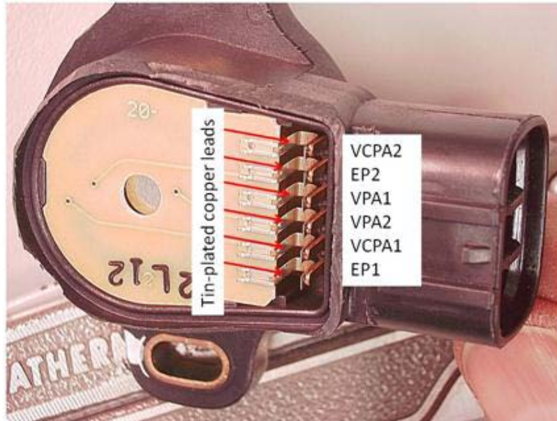
Figure 6.6.2.3-5. Disassembled Accelerator Pedal Assembly Potentiometer
