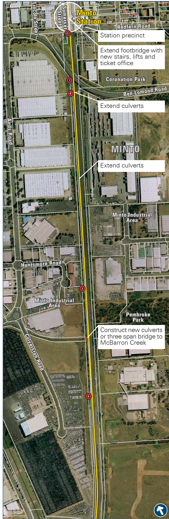
Figure 4.1b Features of corridor construction
