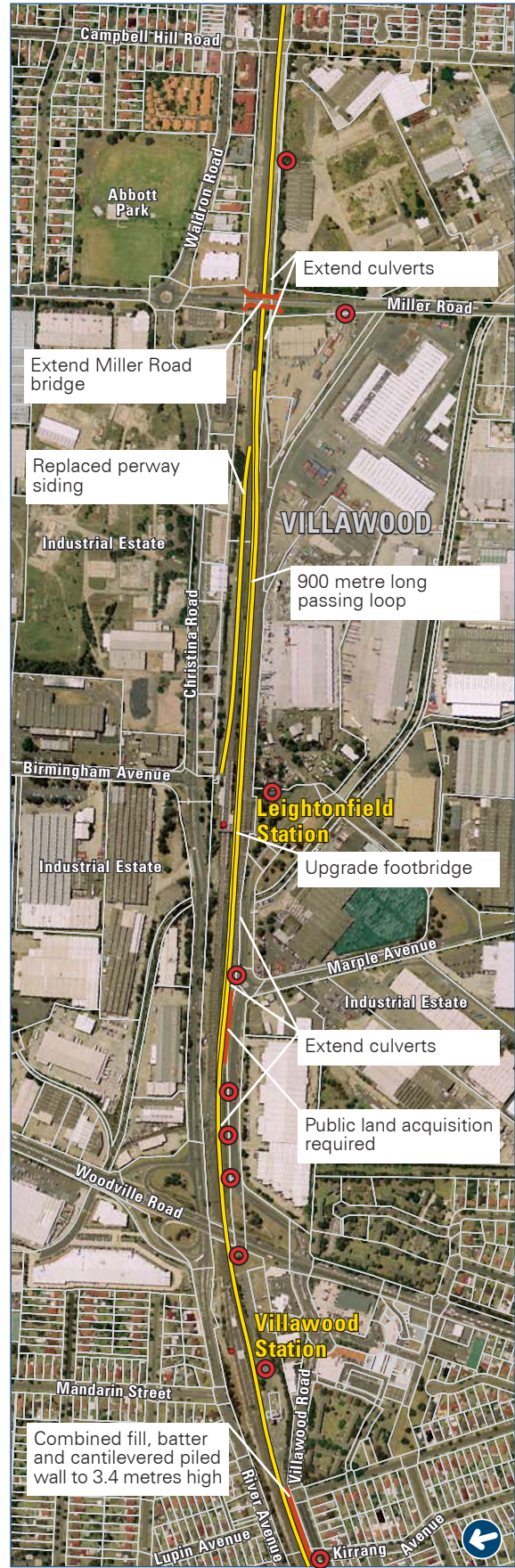
Figure 4.1g Features of corridor construction
