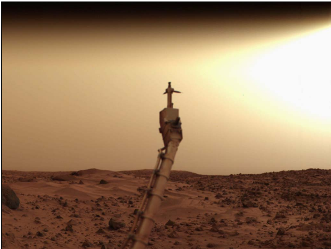
Figure 5. The Viking landers transmitted images using three separate filters, red, green and blue. This negated the need for creating an intermediate channel. The three images were processed to reduce noise and line dropouts and then combined. The colours in the resulting image were tweaked to accurately portray the colours of a Martian sunset.
