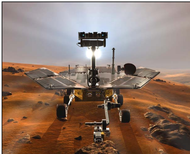
Figure 8. The Martian sun rises over the Opportunity Mars Exploration Rover (MER). The sun will soon rise high enough to provide enough power for the solar panelled rover, lying dormant during the night, to wake up. The rover and elements within the scene were modelled in 3D and are based on actual spacecraft photographs from NASA.
