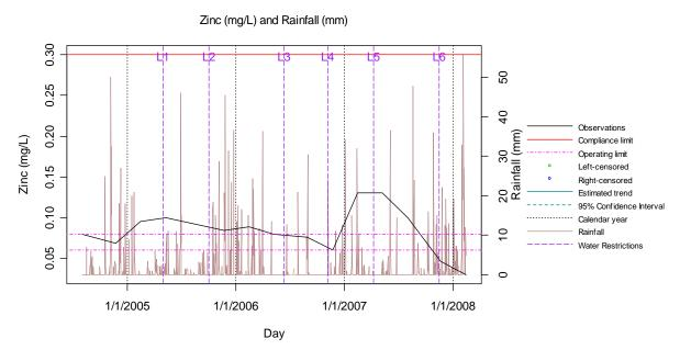
Figure 36 Plot of Effluent Zinc Levels Recorded at Bundamba WWTP
