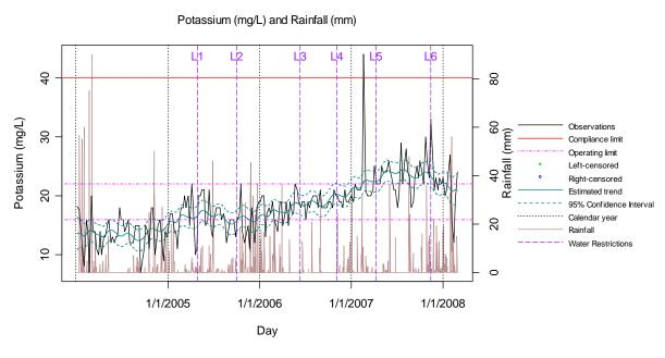
Figure 31 Plot of Effluent Potassium Levels Recorded at Bundamba WWTP
