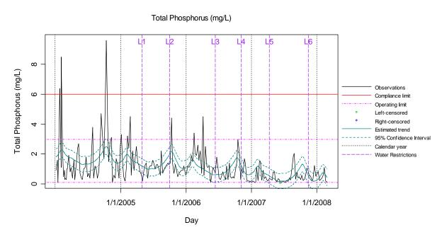
Figure 20 Plot of Effluent Total Phosphorus Values Recorded at Bundamba WWTP
