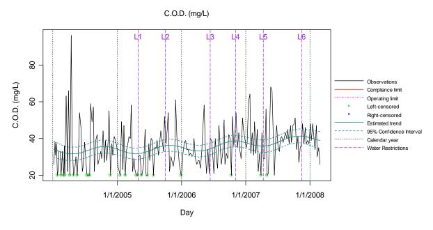
Figure 22 Plot of Effluent COD Values Recorded at Bundamba WWTP
