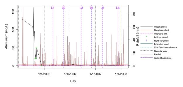
Figure 38 Plot of Effluent Aluminium Levels Recorded at Bundamba WWTP
