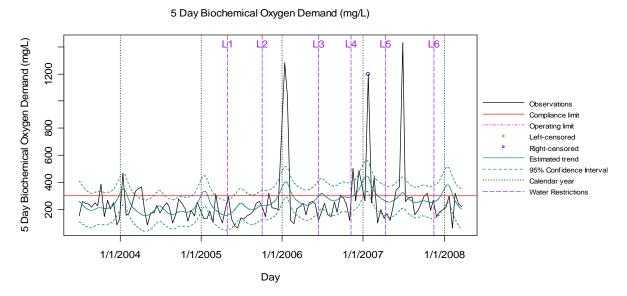
Figure 3 Observed Raw Influent BOD<sub>5</sub> Levels Over Time
