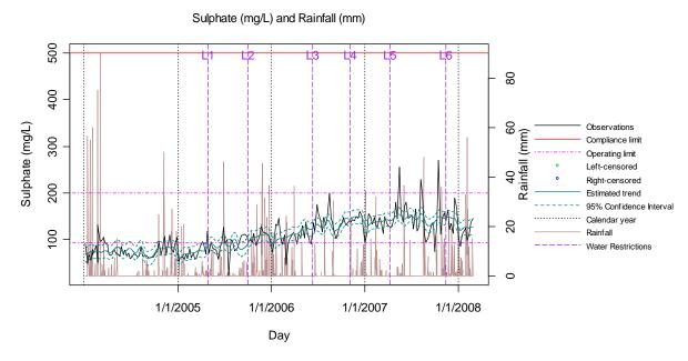
Figure 28 Plot of Effluent Sulphate Levels Recorded at Bundamba WWTP
