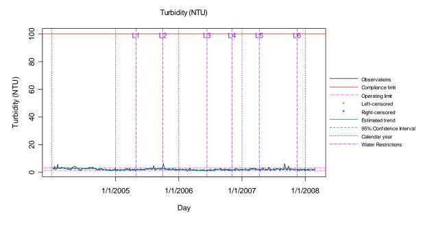
Figure 14 Plot of Effluent Turbidity Recorded at Bundamba WWTP
