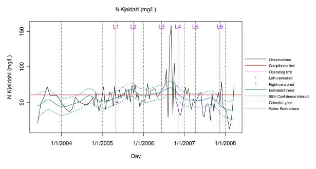
Figure 4 Observed Influent Total Kjeldahl Nitrogen Levels
