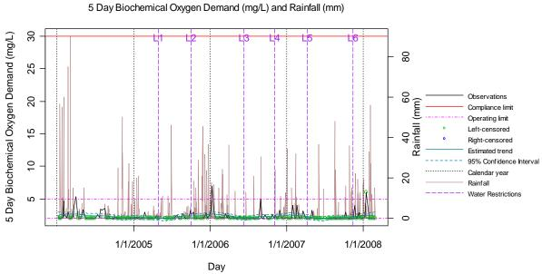
Plot of Effluent BOD<sub>5</sub> Values Recorded at Bundamba
