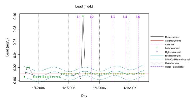
Figure 48 Plot of the Lead Values Recorded at Marburg Delivery Point
