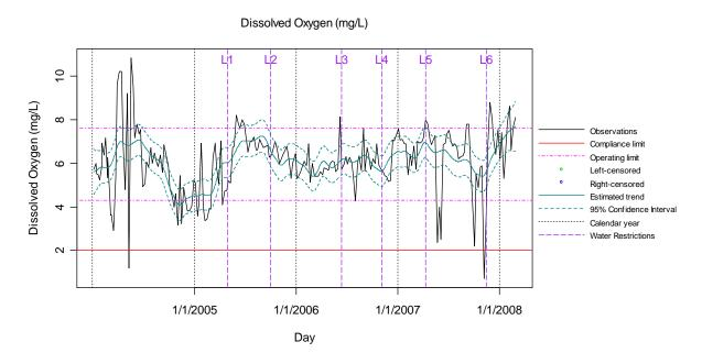
Figure 16 Plot of Effluent DO Levels Recorded at Bundamba WWTP
