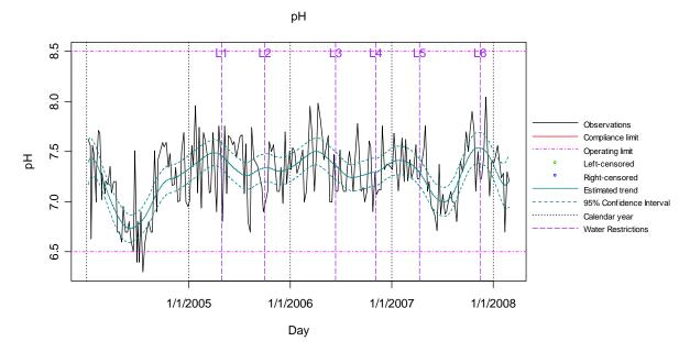
Figure 12 Plot of Effluent pH Recorded at Bundamba WWTP
