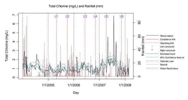
Figure 25 A Plot of Effluent Total Chlorine Levels Recorded at Bundamba WWTP
