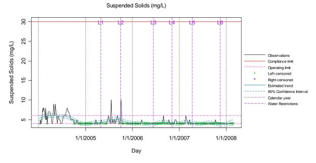
Figure 15 Plot of Effluent Suspended Solids Levels Recorded at Bundamba WWTP
