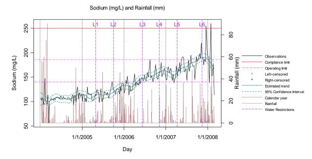
Figure 30 Plot of Effluent Sodium Levels Recorded at Bundamba WWTP
