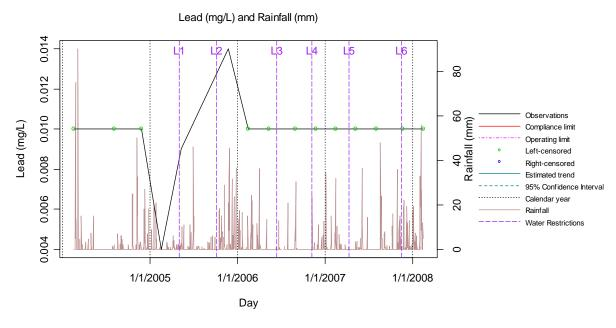
Figure 34 Plot of Effluent Lead Levels Recorded at Bundamba WWTP
