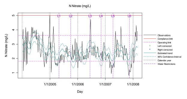
Figure 18 Plot of Effluent Nitrate (as N) Values Recorded at Bundamba WWTP
