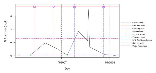
Figure 17 Plot of Effluent Ammonia (as N) Values Recorded at Bundamba WWTP
