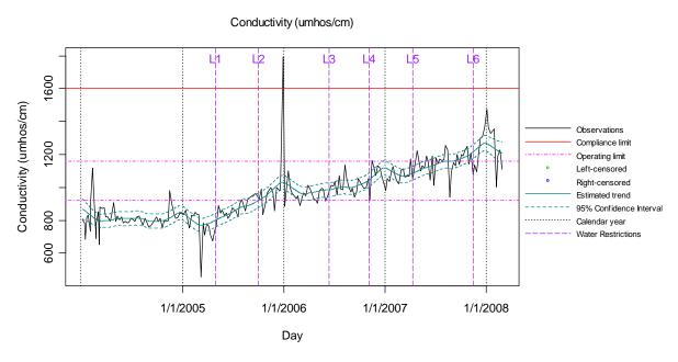
Figure 13 Plot of Effluent Conductivity Recorded at Bundamba WWTP
