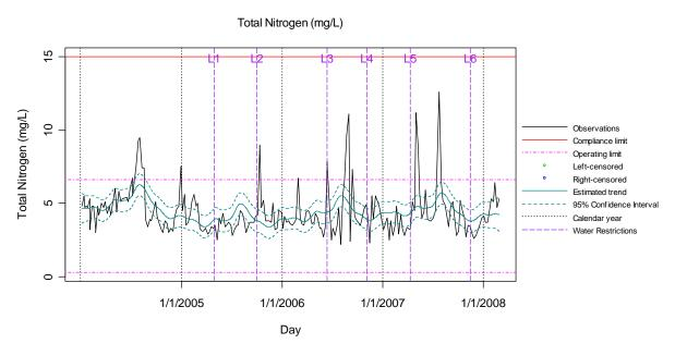
Figure 19 Plot of Effluent Total Nitrogen Values Recorded at Bundamba WWTP
