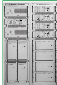
VHF UHF combi module with Series 800 multi-channel transmitters and Agon Multicoupler F0221WA (400 MHz and F0221 VWA (200 MHz)
