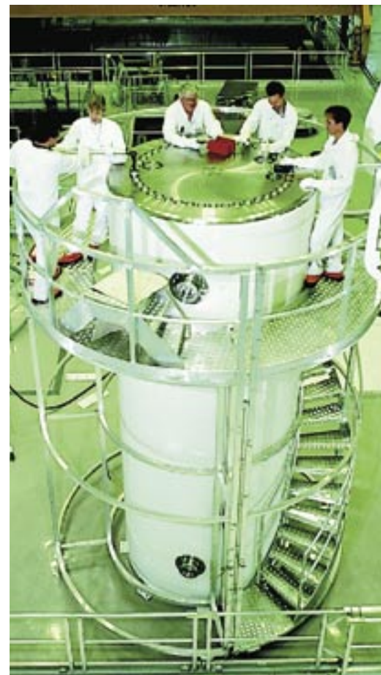
A transport cask for spent nuclear fuel in Olkiluoto.
